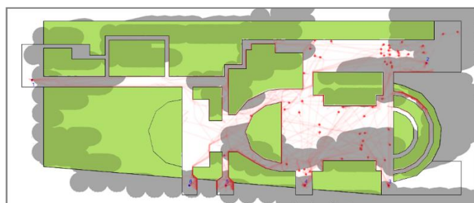
Figure 11. Paths of agents on the spring equinox day at 4 p.m.
