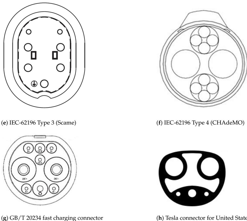
**Figure 7.** EV Connectors considered by the different standards [77–79].
