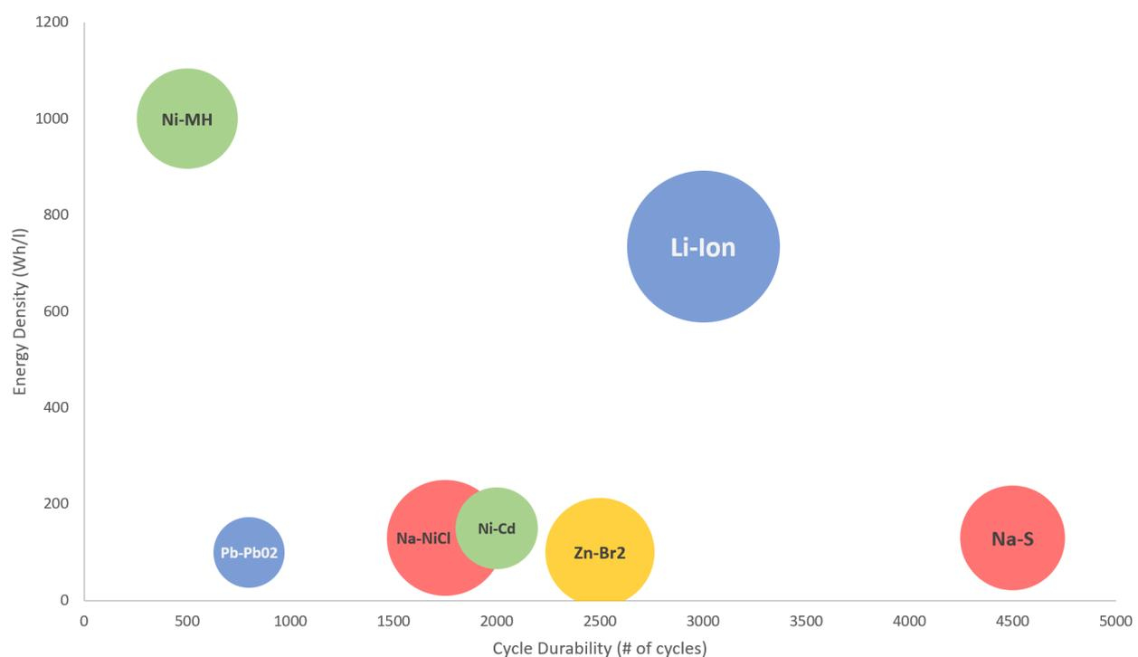
**Figure 6.** A comparison of battery technologies in terms of their Cycle Durability (x-axis), Energy Density (y-axis), Specific Energy (bubble size), and Working Temperature (bubble color). Note that warm colors represent higher working temperatures.
