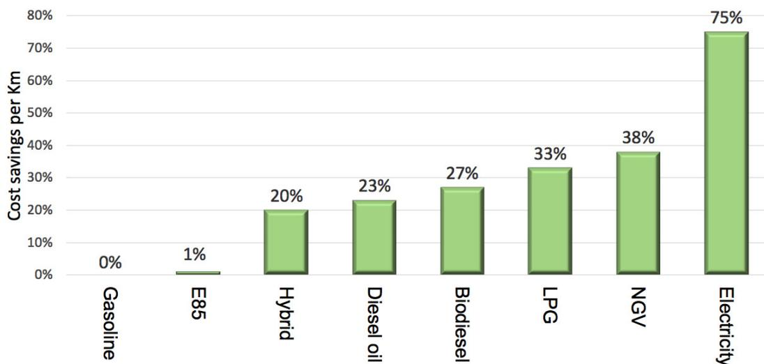
**Figure 1.** Comparison of savings in cost per kilometer offered by vehicles powered by Gasoline, Ethanol (E85), Hybrid, Diesel oil, Biodiesel, Liquefied Petroleum Gas (LPG), Natural Gas Vehicle (NGV), and Electricity [5].
