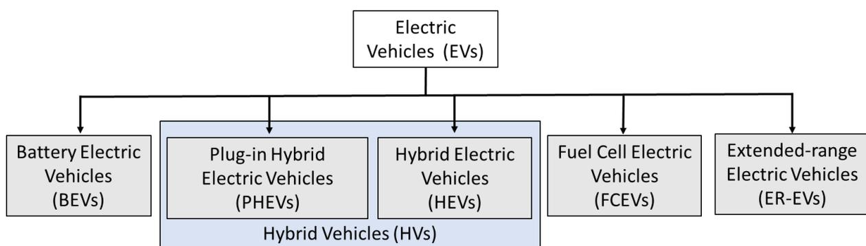
**Figure 3.** Electric vehicles classification according to their engine technologies and settings.
