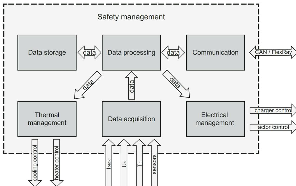
**Figure 8.** Main components of the Battery Management System (BMS) [87].
