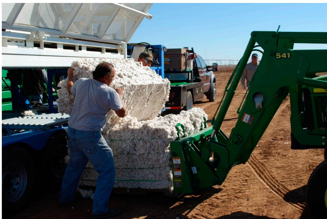
**Figure 1.** Custom weigh cart/micro-module builder for field trials in cotton harvesting research. The system runs off a generator and houses critical field instrumentation for weighing modules and measuring moisture content.
