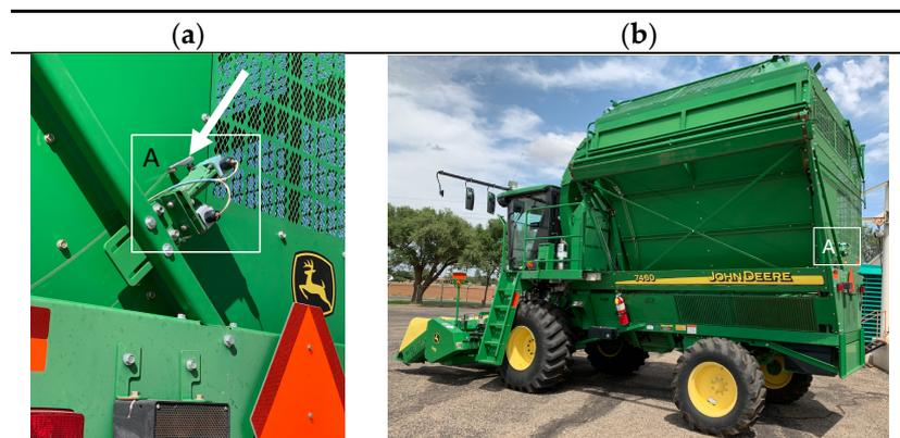
**Figure 2.** Pictures showing the mounting location of the two limit switches, inset box A in both images, that let the micro-controller know when the basket is in the weigh position. The arrow in image (a) is pointing to the roller arm on the second, final destination, limit switch that senses when the basket passes this location and has arrived at its target weighing height. (b) harvester.
