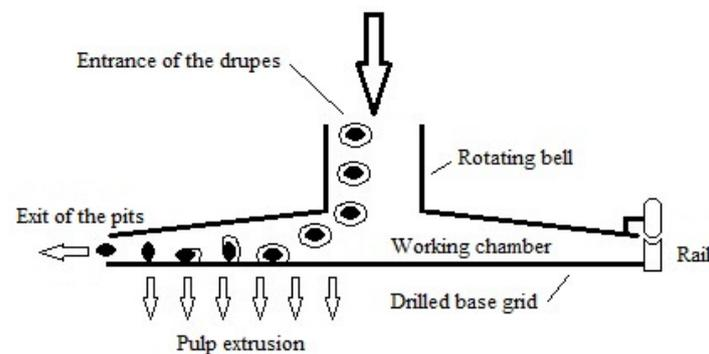
Figure 1. Conceptual scheme of the pitting prototype.
