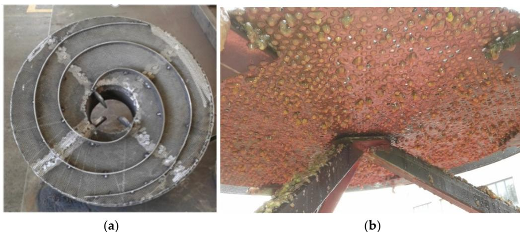
**Figure 5.** Third prototype realisation: (a) double spiral working chamber; (b) extrusion of pitted olive pulp.
