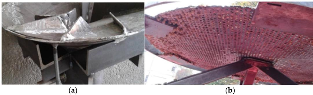
**Figure 4.** Second prototype realisation: (a) working chamber with multiple tangential straight wings; (b) extrusion of pitted olive pulp.
