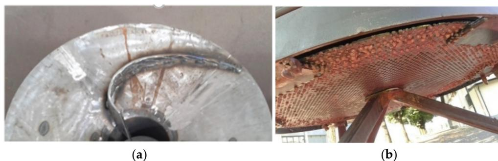
**Figure 3.** First prototype realisation: (a) working chamber with 3 spiral blades; (b) extrusion of pitted olive pulp.
