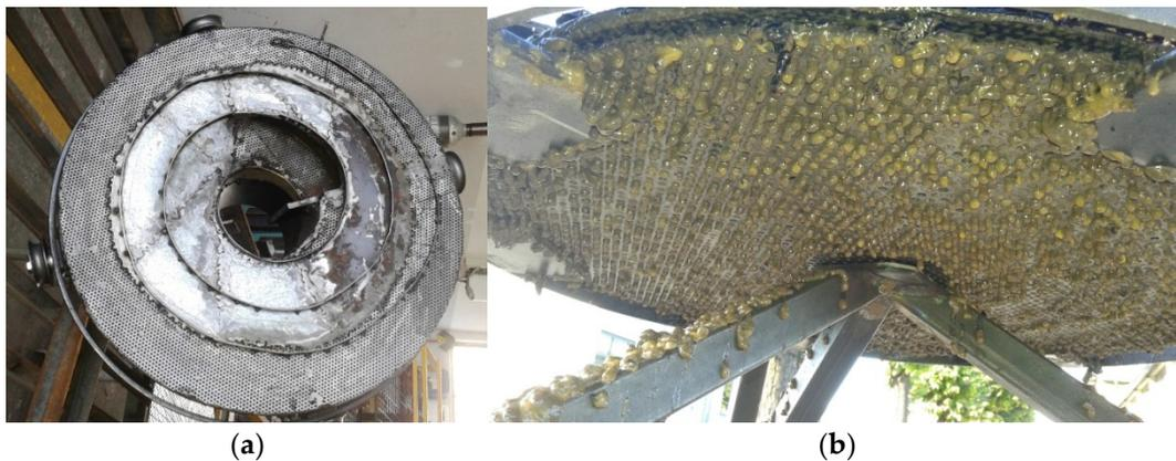
**Figure 6.** The final prototype: (a) collection chamber below the feed window and a single spiral conveyor bulkhead working chamber; (b) extrusion of pitted pulps.
