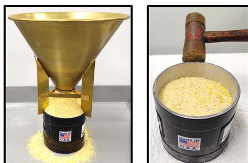
**Figure 1.** Ground grain emptying into standard container from the discharge funnel (left). Tapping procedure to achieve tapped density (right).
