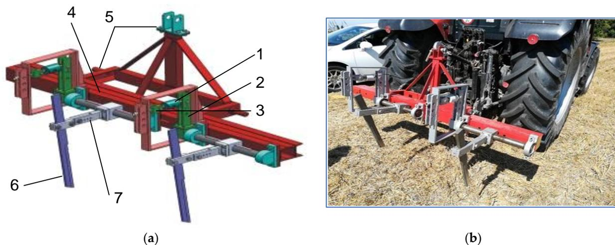
**Figure 2.** Measuring instrument. (a) Measuring instrument with two-element comparison method 1—power sensor EMS 150, 2—arm, 3—attachment to the power sensor, 4—frame, 5—attachment of the three-point hitch, 6—blade, 7—blade clutch. (b) Measurement of the horizontal soil resistivity in comparative measurements.
