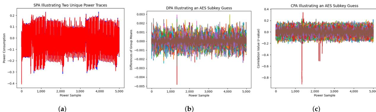
**Figure 1.** Visualizations for Simple Power Analysis (SPA), Differential Power Analysis (DPA), and Correlation Power Analysis (CPA) that accompany the methodological discussions in Section 2. (a) Sample SPA visualization. (b) Sample DPA visualization. (c) Sample CPA visualization.
