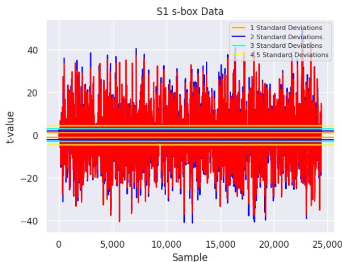
**Figure 2.** An example TVLA output for fixed and random plaintext outputs when run through Tiny-AES-c with the S1 s-box.
