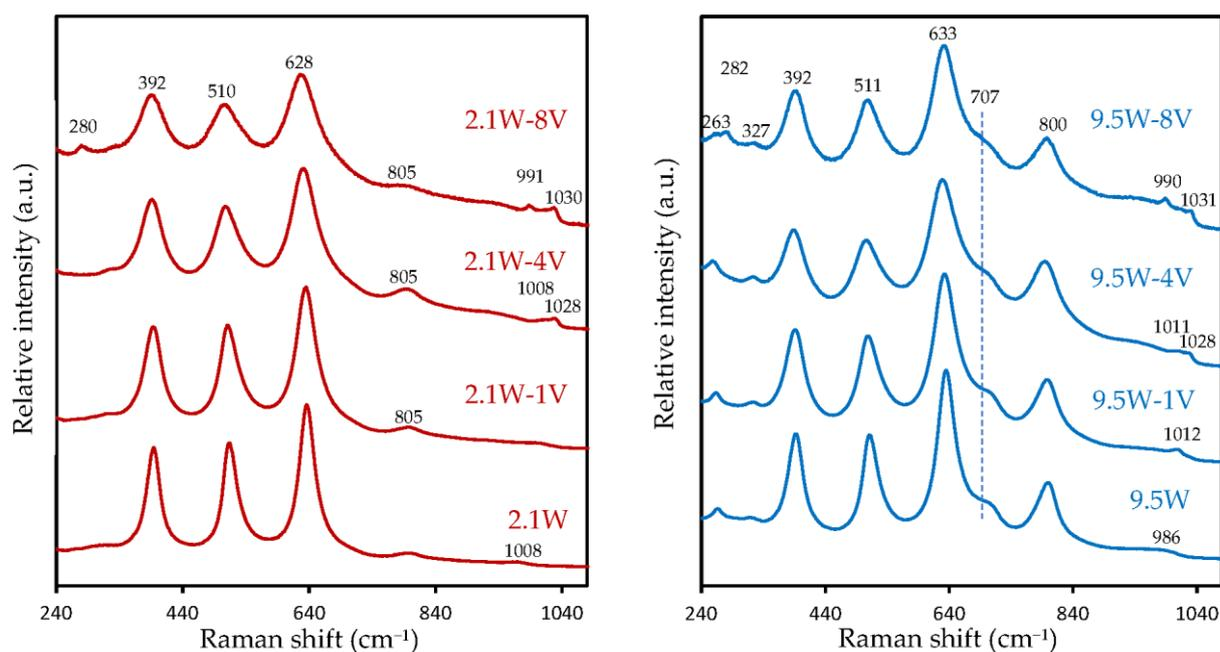
**Figure 6.** Raman spectra recorded on  $\text{V}_2\text{O}_5\text{-WO}_3/\text{TiO}_2$  catalysts calcined in air at  $450\text{ }^\circ\text{C}$ .
