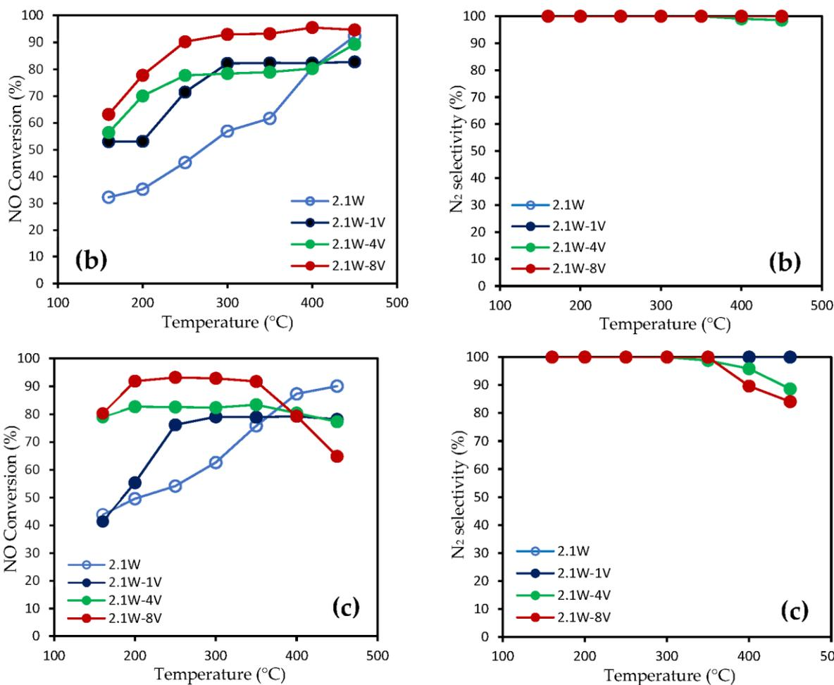
**Figure 2.** Conversion and N<sub>2</sub> selectivity profiles vs. temperature recorded on 2.1W-xV during ammonia SCR: (a) Dry ID 2 operating conditions on preheated freshly prepared samples; (b) Wet conditions ID 3; (c) Dry conditions ID 2 on samples exposed to wet conditions according to ID3. Gas hourly space velocity of 75,000 mL.h<sup>-1</sup>.g<sup>-1</sup>.
