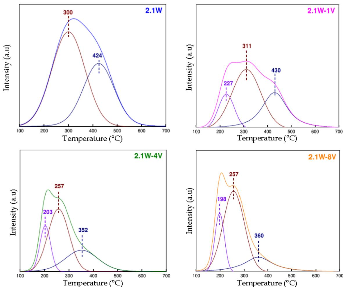
**Figure 10.** Normalized ammonia-TPD profiles recorded for 2.1W- $x$ V: impact of V loading on the acidic functionality.
