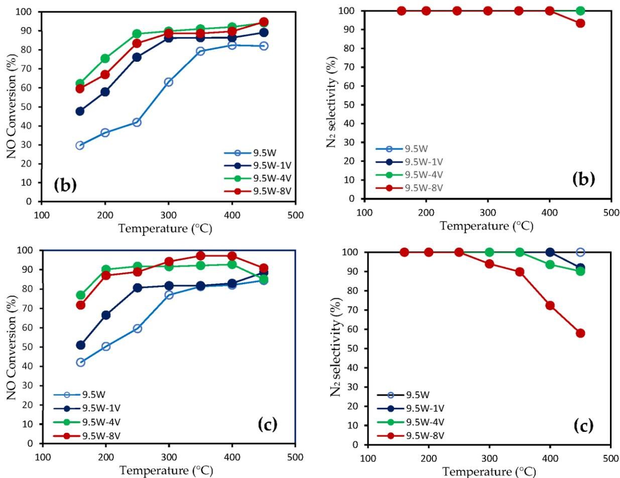
**Figure 3.** Conversion and  $N_2$  selectivity profiles vs. temperature recorded on 9.5W- $x$ V during ammonia SCR: (a) Dry ID 2 operating conditions on preheated freshly prepared samples; (b) Wet conditions ID 3; (c) Dry conditions ID 2 on samples exposed to wet conditions according to ID3. Gas hourly space velocity of  $75,000 \text{ mL}\cdot\text{h}^{-1}\cdot\text{g}^{-1}$ .
