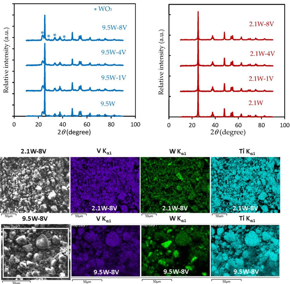
**Figure 5.** XRD and EDS analyses on freshly prepared V<sub>2</sub>O<sub>5</sub>-WO<sub>3</sub>/TiO<sub>2</sub> catalysts calcined in air at 450 °C.
