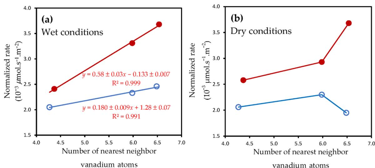
**Figure 11.** Dependency of the nearest vanadium atoms in  $\text{VO}_x$  clusters on the normalized reaction rates measured on 2.1W- $x$ V (○) and 9.5W- $x$ V (●) exposed at 160 °C to 400 ppm NO, 400 ppm  $\text{NH}_3$ , 8 vol.%  $\text{O}_2$  in the presence (a) and in the absence of 10 vol.%  $\text{H}_2\text{O}$  (b).
