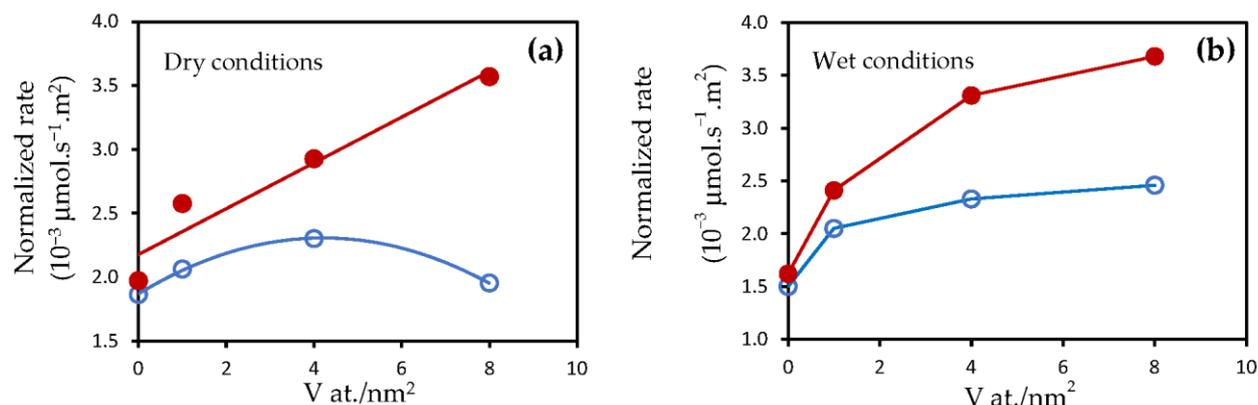
**Figure 4.** Vanadium density and relative concentration of vanadium dependencies of the normalized reaction rate of 2.1W- $x$ V (○) and 9.5W- $x$ V (●) in ammonia-SCR: 400 ppm NO, 400 ppm NH<sub>3</sub>, 8 vol.% O<sub>2</sub> in the presence (wet conditions) or in the absence (dry conditions) of 10 vol.% H<sub>2</sub>O: (a) dry conditions; (b) wet conditions.
