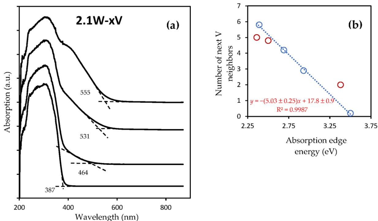
**Figure 7.** UV-vis spectra recorded for the series 2.1W- $x$ V (a) and relationship between the estimated absorption edge value from (a) and the number of next V neighbors in  $\text{VO}_x$  clusters (b). Red circle data from reference [27], blue circle data from reference [28].
