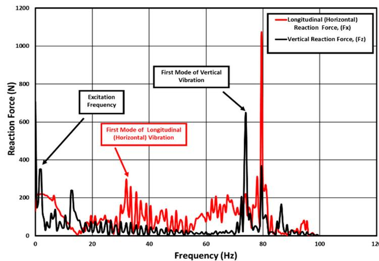
**Figure 8.** Frequency analysis of a 235/55R19 tire at 228 kPa inflation pressure and 5 kN vertical load.
