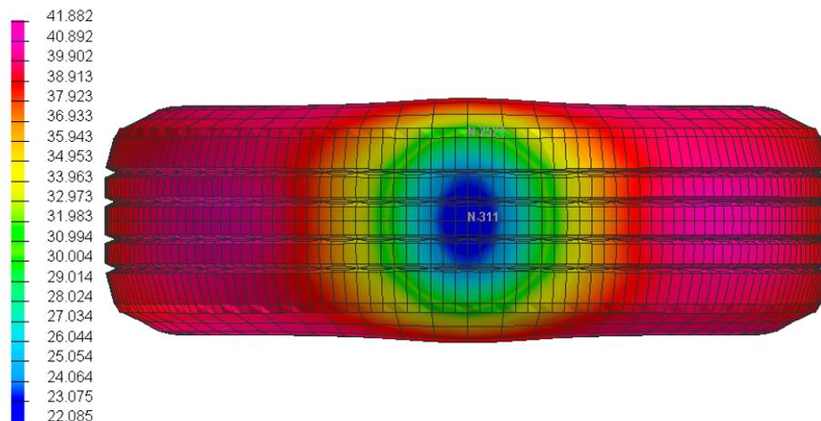
**Figure 6.** The nodal displacement contour at footprint test for nominal inflation pressure and nominal load.
