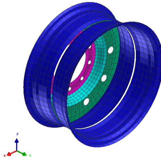
**Figure 3.** Aluminum wheel assembly FEA model in Pam-Crash software.
