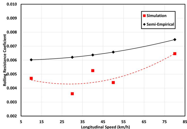
**Figure 11.** RRC as a function of five longitudinal speeds (10 km/h, 30 km/h, 40 km/h, 50 km/h, and 80 km/h) at 228 kPa inflation pressures and an 8 kN vertical load.
