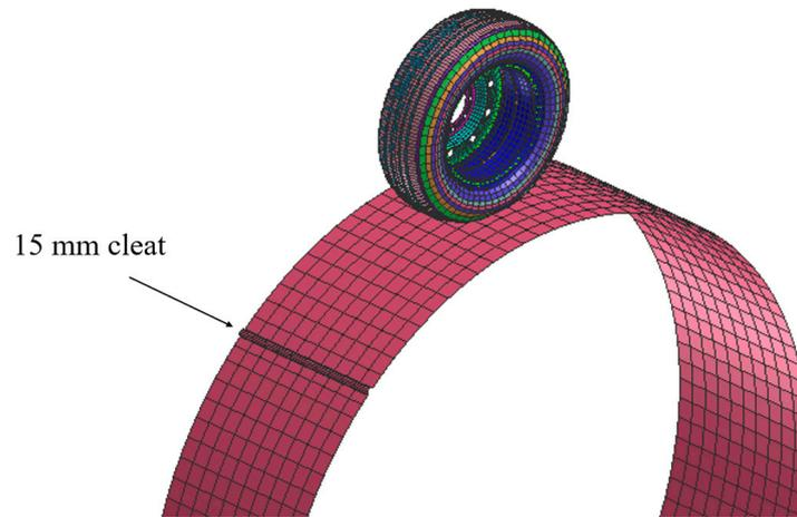
**Figure 7.** Tire drum-cleat test setup for the FEA passenger car tire model.
