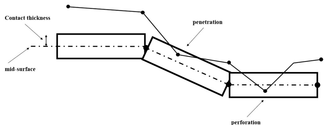
**Figure 4.** Contact definition in Pam-Crash, perforation, and penetration [25].
