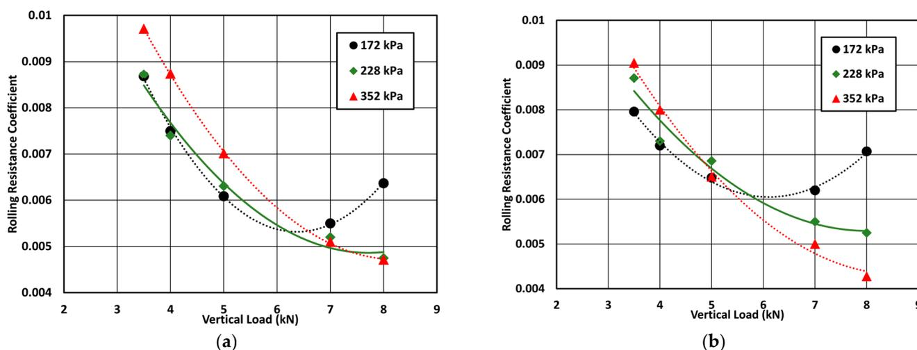
Figure 9. Tire RRC as a function of vertical load at three inflation pressures and longitudinal speeds: (a) 10 km/h longitudinal speed; (b) 40 km/h longitudinal speed.
