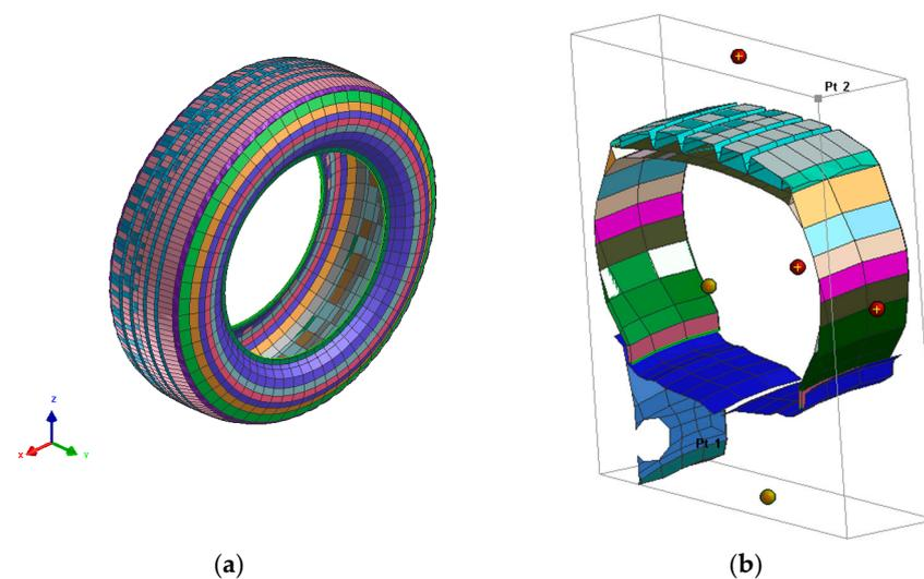
Figure 2. FEA 235/55R19 tire in Pam-Crash. (a) FEA full rotated tire; (b) cross-section of the tire.
