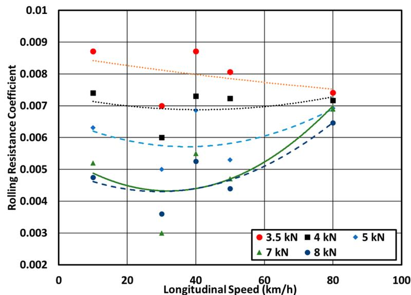
Figure 10. Effect of longitudinal speed on the tire's rolling resistance coefficient at different vertical loads and a nominal inflation pressure of 228 kPa.
