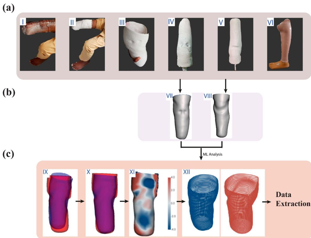
**Figure 1.** The workflow for evaluating the correction procedure in this study: (a) typical socket manufacturing process followed by BMVSS; (b) three-dimensional laser-scanned unmodified and modified casts; (c) stages of the shape analyses toolbox from misaligned surface scans to pairwise cast quantification.
