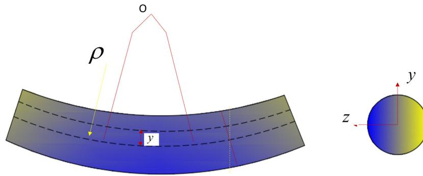
**Figure 6.** Shaft deformation under elastoplastic bending.
