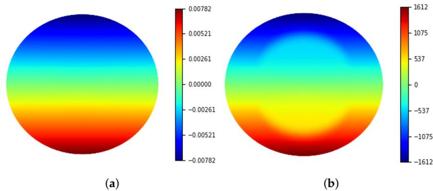
Figure 8. Stress and strain distribution at the location of loading: (a) strain distribution; (b) stress [MPa] distribution.
