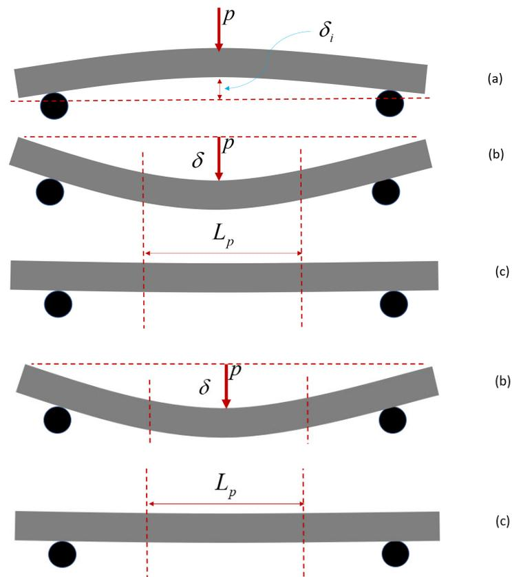
**Figure 1.** Illustration of the shaft bend straightening process: (a) distorted shaft to be straightened; (b) shaft deflected under straightening load; (c) straightened shaft.
