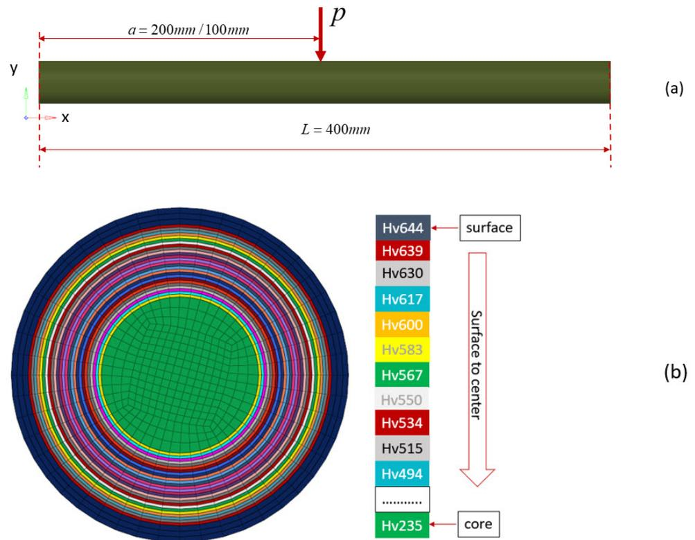
**Figure 12.** Finite element model: (a) overall dimensions; (b) cross-section of layered finite element model with hardness mapping.
