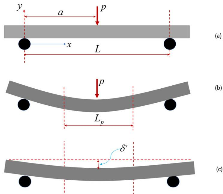
**Figure 2.** Analytically modeled straightening process: (a) an ideally straight shaft subjected to a bending load; (b) deflected shaft under load; (c) unloaded shaft with residual deflection.
