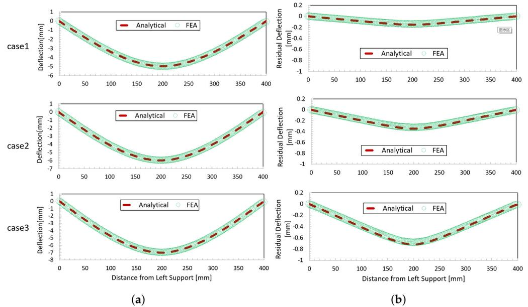
**Figure 13.** Shaft deflections for the load applied in the middle of shaft cases 1–3: (a) shaft deflection under loading; (b) residual deflection.
