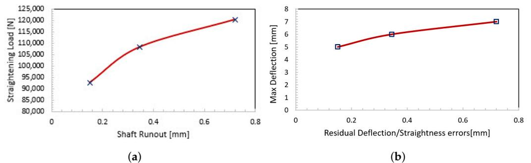
**Figure 15.** Plots of straightening load and stroke displacement in terms of residual deflection: (a) straightening load vs. residual deflection; (b) stroke displacement vs. residual deflection.
