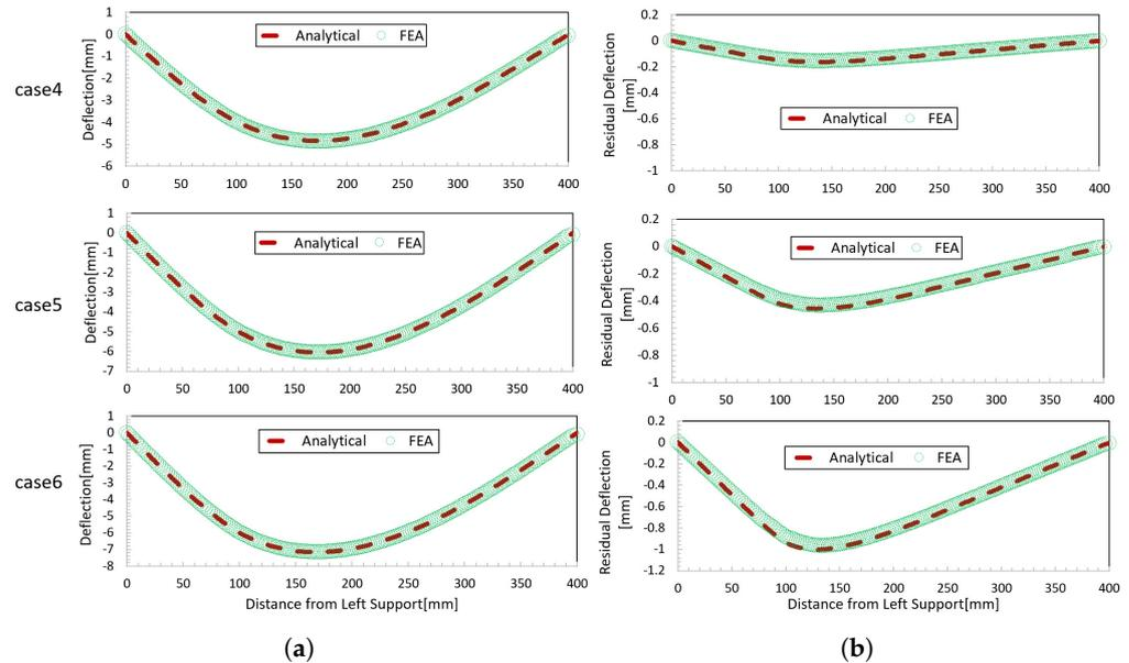
**Figure 14.** Shaft deflections for load applied at the quarter of shaft cases 4–6: (a) shaft deflection under loading; (b) residual shaft deflection.
