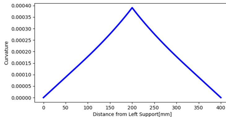
**Figure 7.** Curvature distribution along shaft axis as loaded.
