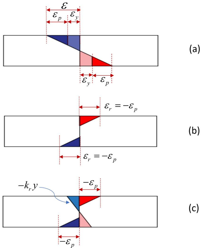
Figure 10. Strain evolution in the straightening process: (a) strain distribution under loading; (b) residual strain distribution without residual deflection; (c) resultant residual strain with residual deflection.
