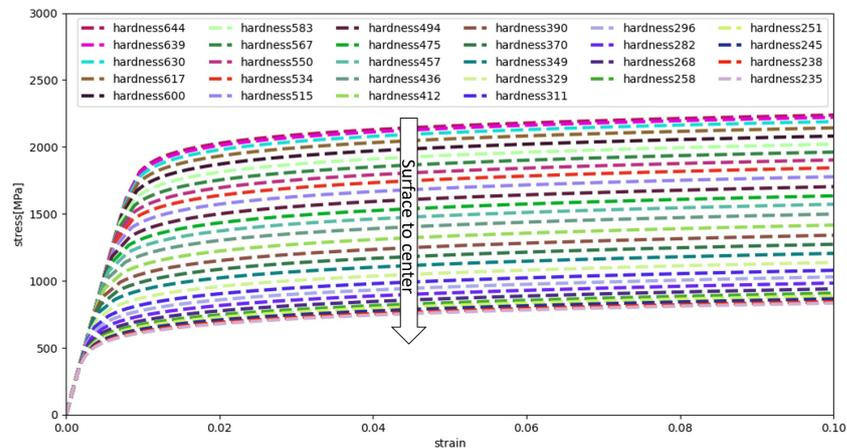
Figure 4. Hardness-based true stress–strain curves.
