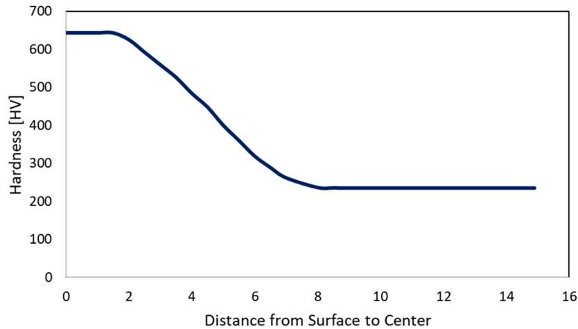
Figure 3. A typical hardness profile resulting from induction hardening.
