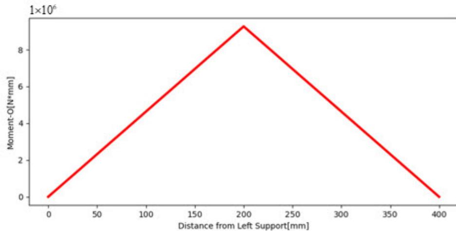
Figure 5. Bending moment diagram.
