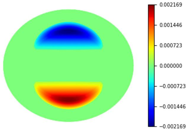
Figure 9. Plastic strain in shaft axial direction.
