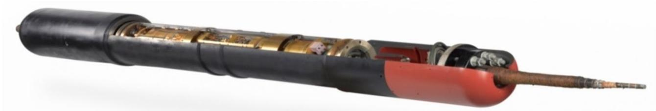
**Figure 16.** First-generation sectioned submerged repeater for TAT-1 the first transatlantic telephone cable [1].
