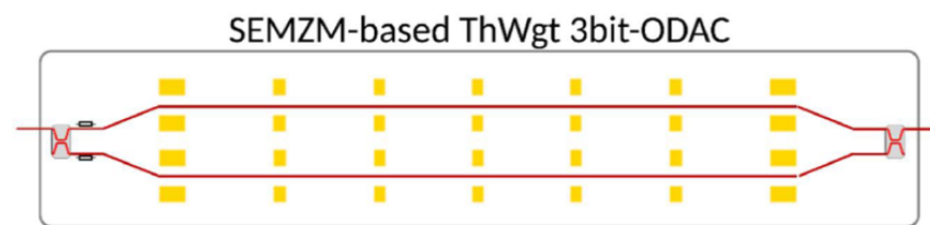
Figure 13. Segmented MZM (SEMZM) 7 segments oDAC architecture-optimized thermometer-weighted DAC Structure for generation of PAM8 signals [22]. This SEMZM comprises seven segments; each segment is described as a yellow box. In red, the optical waveguide that light passes through and is modulated by each segment appropriately is shown.
