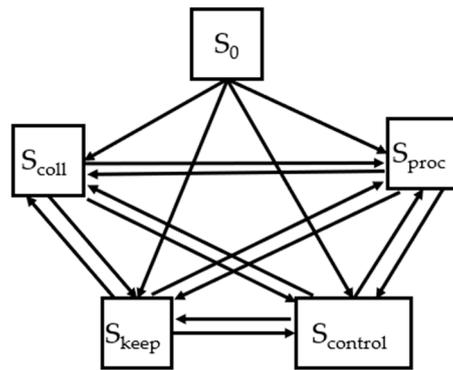
Figure 3. State and transition graph illustrating possible states of a WSN node.
