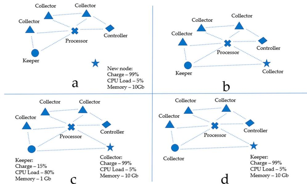
**Figure 8.** Illustration of a self-organizing decentralized WSN operation in the case of (a) new node appearing, (b) assigning a role to a new node, (c) initiating a redistribution of roles and (d) redistributing roles in the network.
