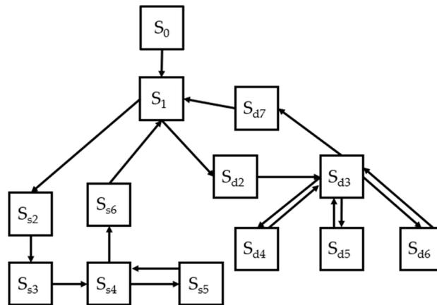
**Figure 2.** State and transition graph illustrating the states of a self-organizing decentralized WSN and transitions between them.
