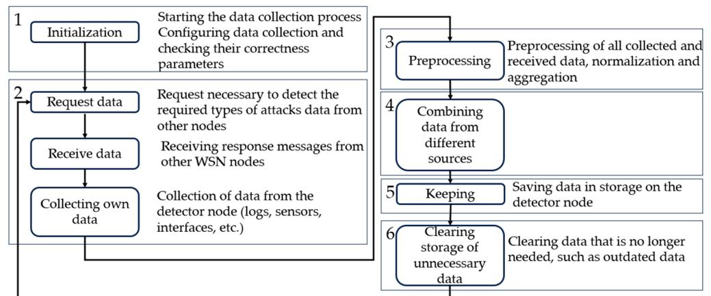
**Figure 5.** Combined data collection algorithm for detecting attacks in WSNs.
