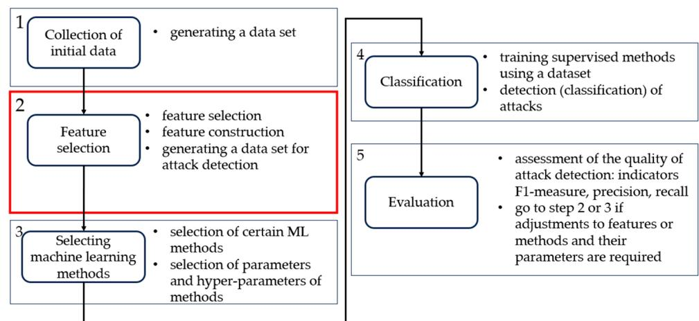
**Figure 6.** Combined algorithm for detecting attacks in WSNs.
