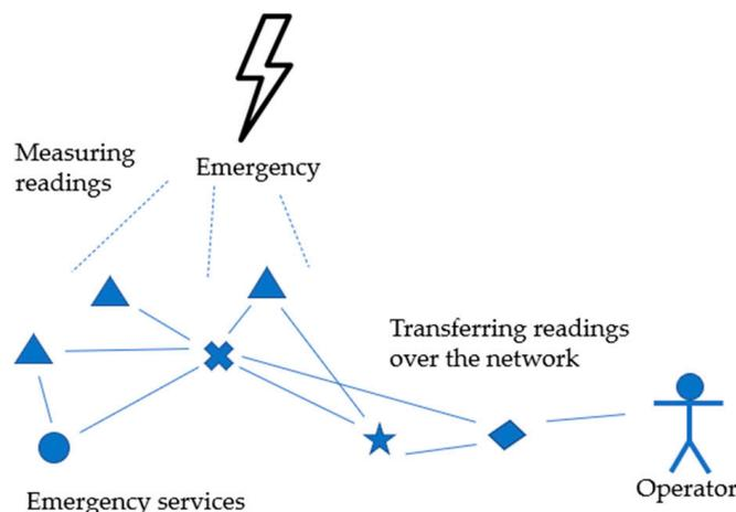
**Figure 1.** An example of a WSN as the element of an anti-crisis response system in emergencies.
