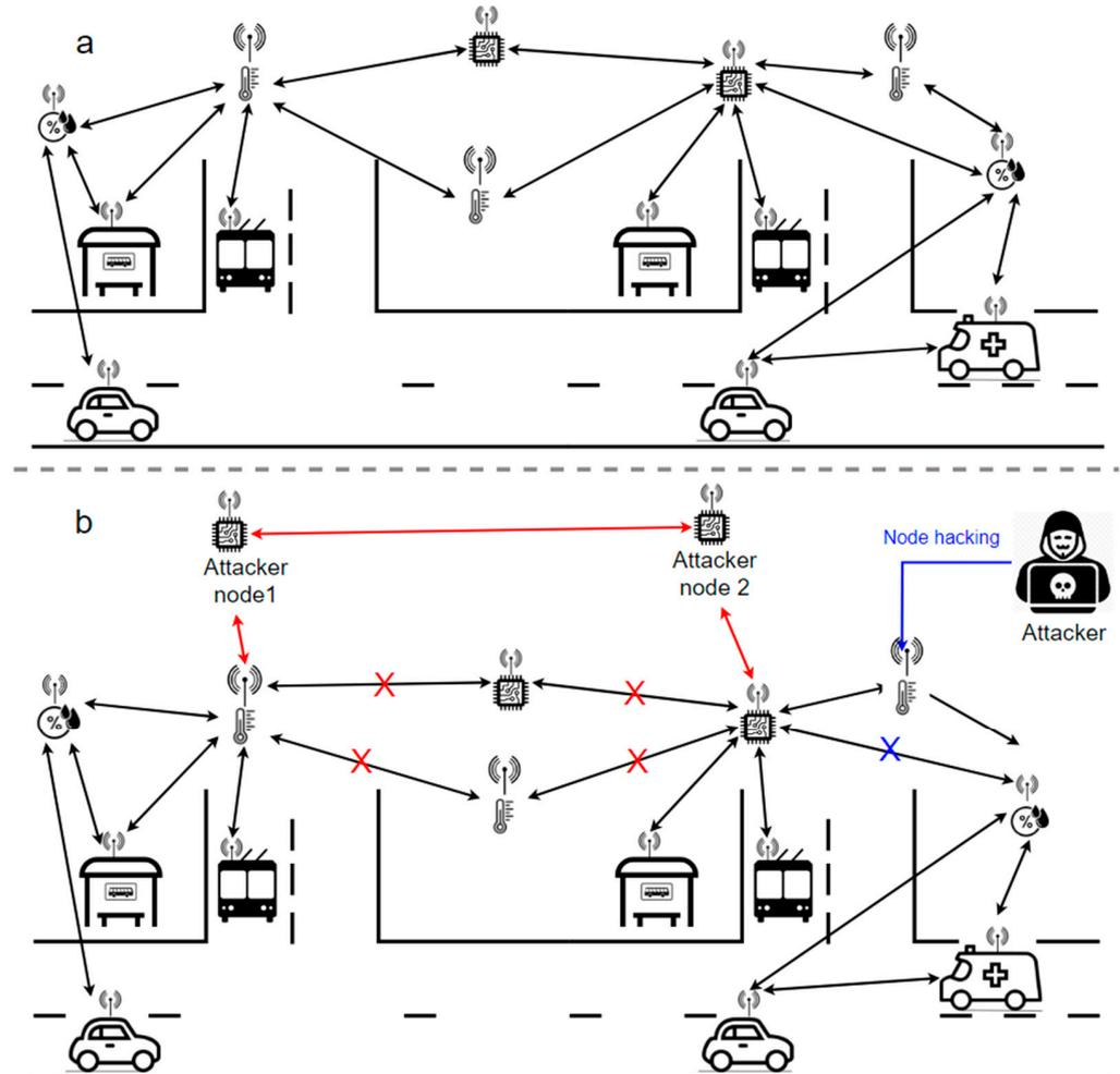
**Figure 4.** Case study of air pollution monitoring example (in an urban infrastructure). (a) Initial WSN indicating the connection between the nodes; (b) WSN under the influence of wormhole and sinkhole attacks.
