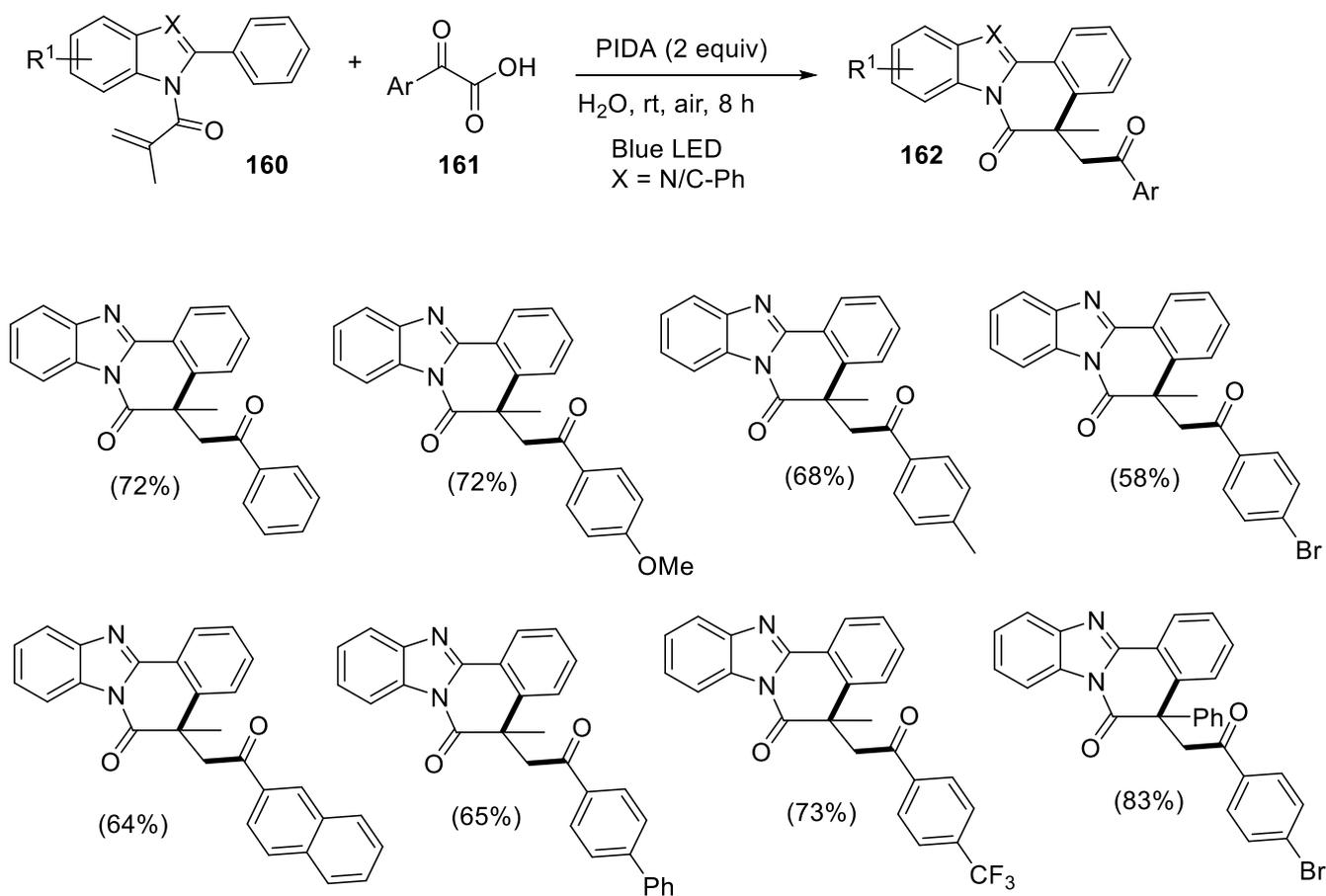
**Scheme 26.** PIDA-mediated metal-free visible-light-induced decarboxylative radical addition/cyclization.
