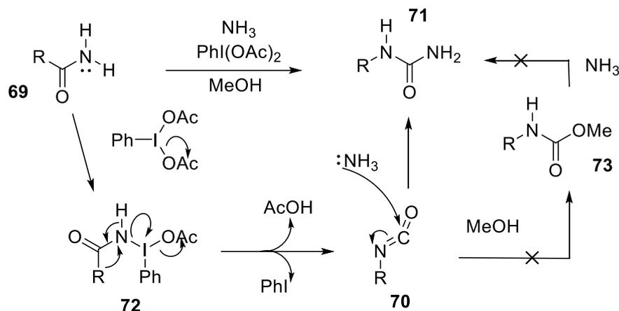
**Figure 11.** Proposed mechanism for PIDA-mediated Hofmann rearrangement.
