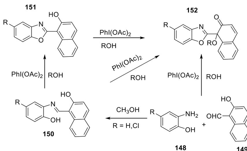
**Scheme 25.** PIDA-mediated oxidation of 2-(2-hydroxynaphthyl)benzoxazoles in alcohols.
