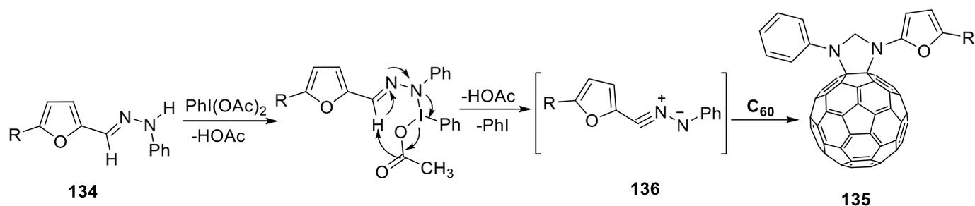
**Figure 19.** Possible mechanism for the formation of furylpyrazolino[60]fullerene derivatives.
