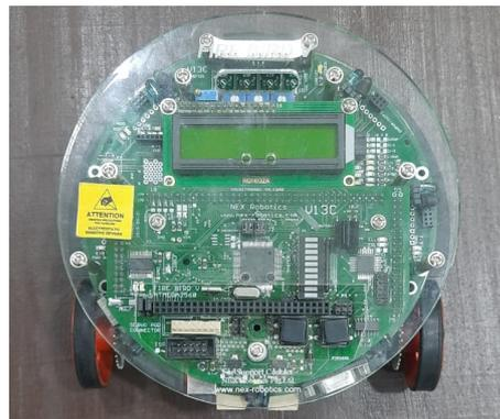
**Figure 6.** Fire Bird V robot.
