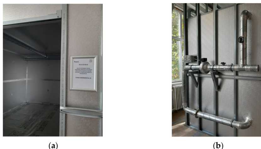
Figure 2. Details of experimental stand for the monitoring of VOC emissions: (a) the experimental stand; (b) the air recirculation installation.
