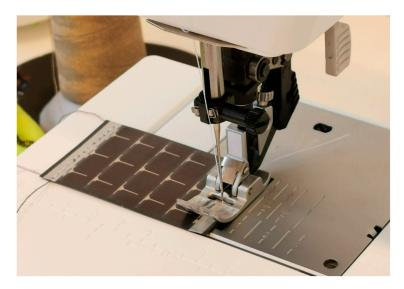
Figure 2. Stitching of flexible solar cells.
