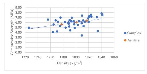
**Figure 4.** Correlation between density and compressive strength for the individual samples (blue dots) and each of the ashlars (orange dots). The linear regression is shown by a dotted blue line.
