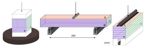
**Figure 2.** Test set ups for the uniaxial compression test (**left**), the three-point bending test (**middle**), and the split test (**right**). The arrow shows the loading direction.
