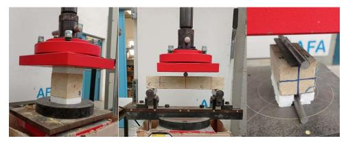
**Figure 3.** Images of the test set up for the uniaxial compression test (**left**), the three-point bending test (**middle**) and split test (**right**).
