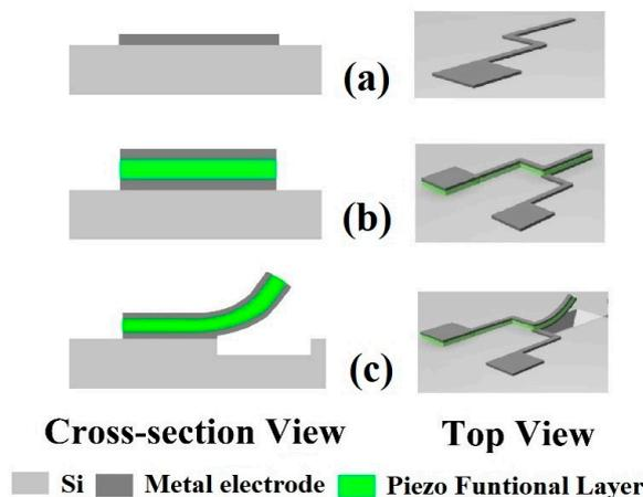
**Figure 3.** Fabrication steps for piezoelectric microcantilever chemical sensor. (a) Bottom electrode patterning. (b) Top electrode patterning for the piezoelectric layer. (c) Release of the cantilever from the Si substrate.
