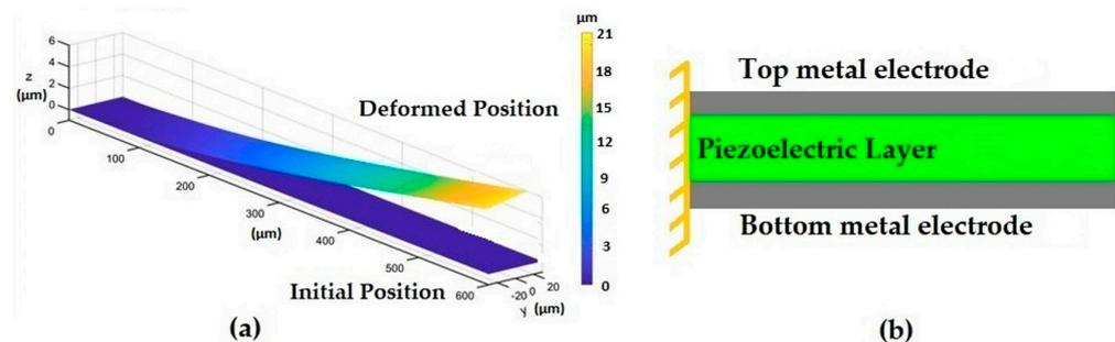
**Figure 1.** (a) Microcantilever simulated in the deformed position. (b) A side view of a microcantilever that was designed.
