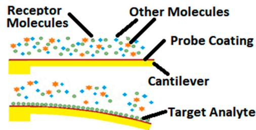
Figure 4. MEMS cantilever bending induced by molecular adsorption.
