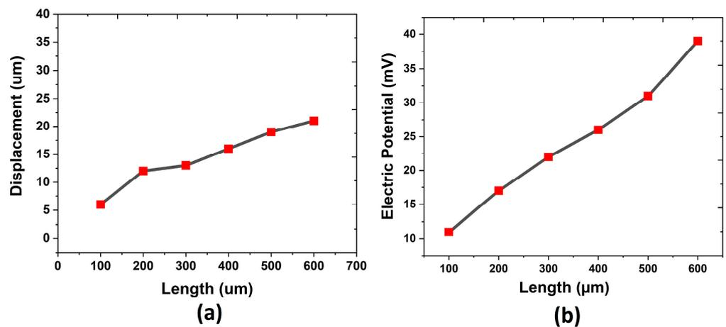
**Figure 2.** (a) Microcantilevers' displacement vs. length. (b) Microcantilevers' electric potential vs. length.
