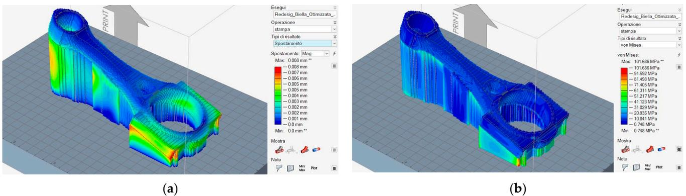
**Figure 7.** (a) Displacement and (b) von Mises stress trends obtained with the printing simulation of the optimized connecting rod.
