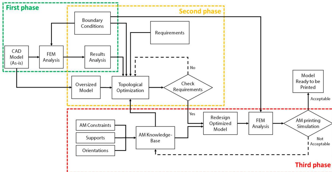
**Figure 2.** Proposed method to optimize the redesign of additive components.
