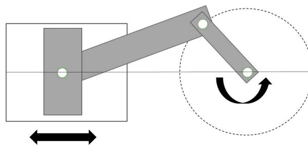
**Figure 1.** Piston-connecting rod–crank system.
