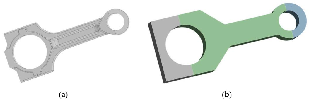
**Figure 3.** (a) CAD model (as-is); (b) oversized CAD model used for the TO analysis.
