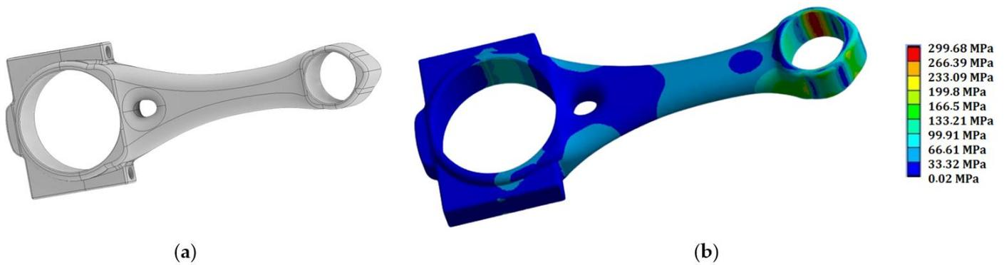
**Figure 6.** (a) Result of the redesign phase; (b) stress distribution—FEM analysis of the worst case (load case 2).
