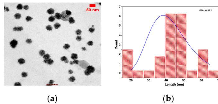
**Figure 4.** (a,b) shows the TEM image and particle size distribution curve of NbSe<sub>2</sub> NPs synthesized via the sonochemical method at room temperature.
