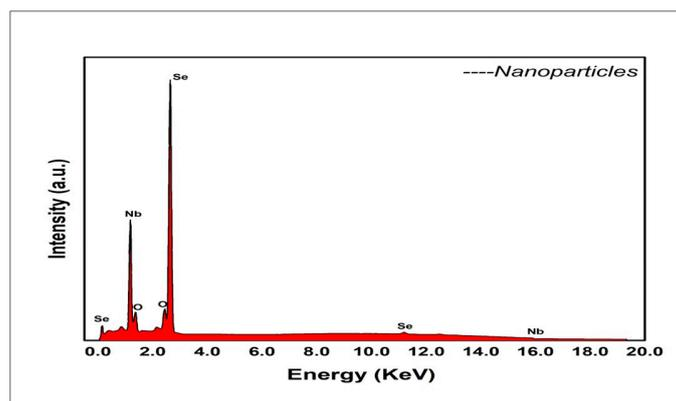
**Figure 1.** The EDS spectrum of NbSe<sub>2</sub> NPs synthesized via sonochemical method at room temperature.
