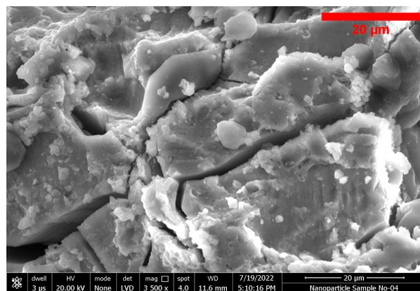
**Figure 3.** The surface morphology SEM image of NPs synthesized via the sonochemical method at room temperature.
