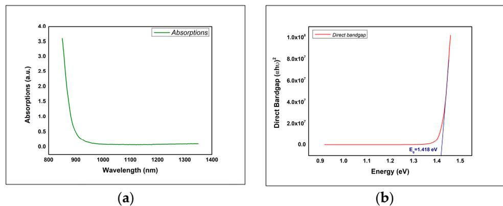
**Figure 5.** (a,b) shows the absorption and optical direct bandgap of NbSe<sub>2</sub> NPs synthesized via the sonochemical method at room temperature.
