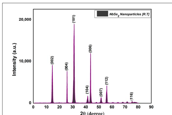
**Figure 2.** The XRD profile of NbSe<sub>2</sub> NPs synthesized via sonochemical method at room temperature.
