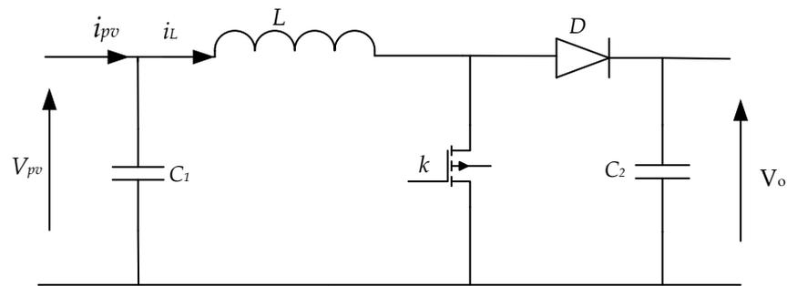
Figure 2. Electrical diagram of DC-DC Boost converter.
