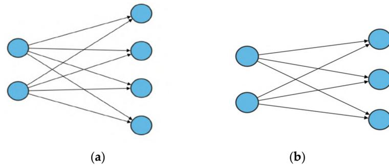
**Figure 2.** Structures of the feedforward artificial neural networks for the classification of corrugated board type for (a) double (5-ply)- or (b) single (3-ply)-walled corrugated boards.
