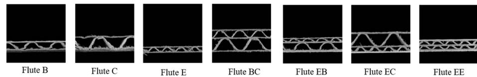
**Figure 1.** Examples of the various corrugated board type cross-sections analyzed in this work.
