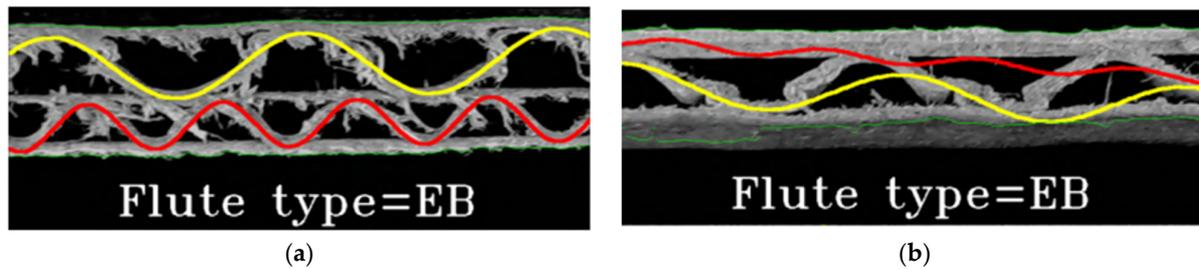
**Figure 5.** Examples of corrugated board samples with (a) jagged edges and cellulose fibers and (b) bent liners.
