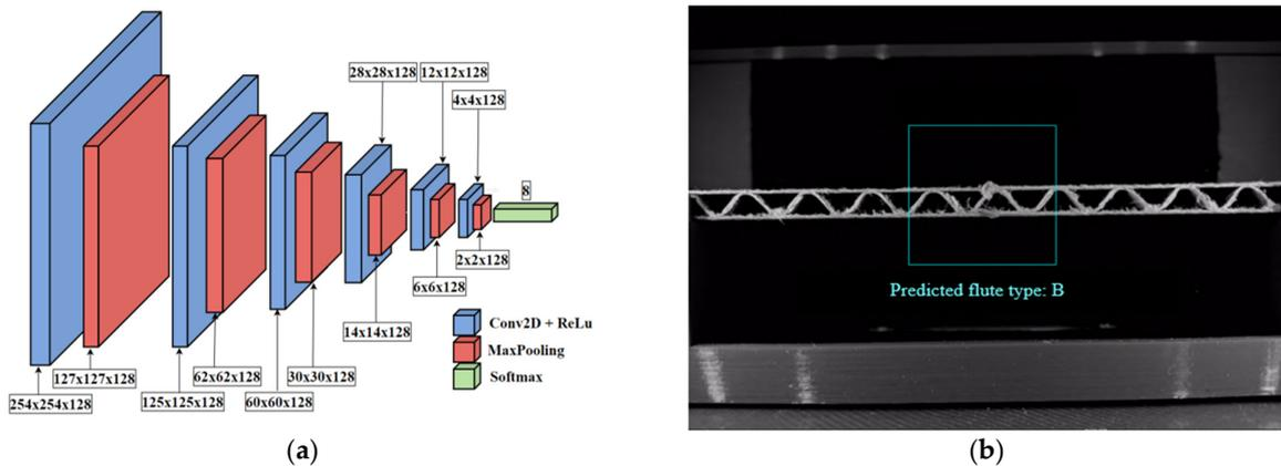
**Figure 3.** (a) The structure of the convolutional neural network applied in this work and (b) the real-time vision system.
