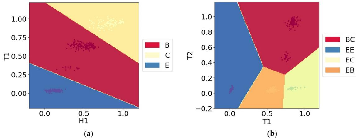
**Figure 4.** Decision boundaries for trained feedforward neural networks designed for (a) single (3 ply)- or (b) double (5 ply)-walled corrugated board.
