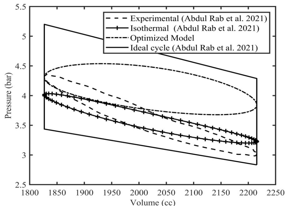
**Figure 1.** Comparison of the optimized model with another thermodynamic model [1].
