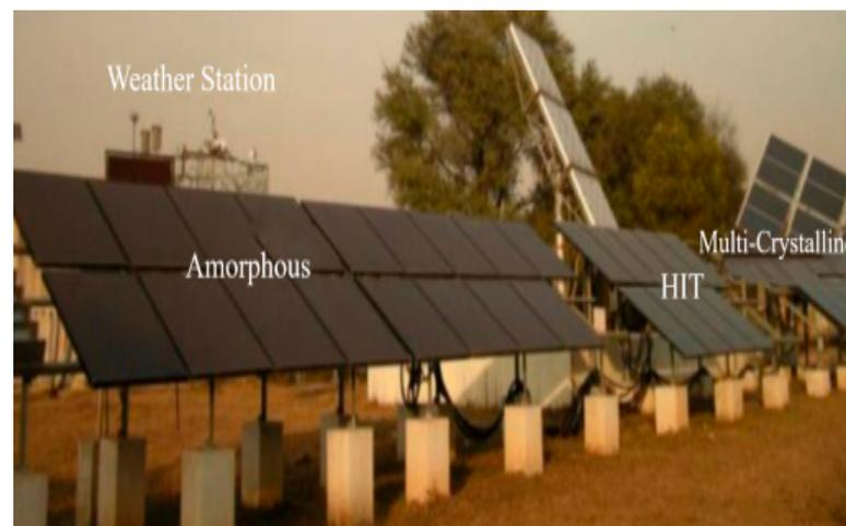
**Figure 1.** Test setup modules at NISE, India [16].
