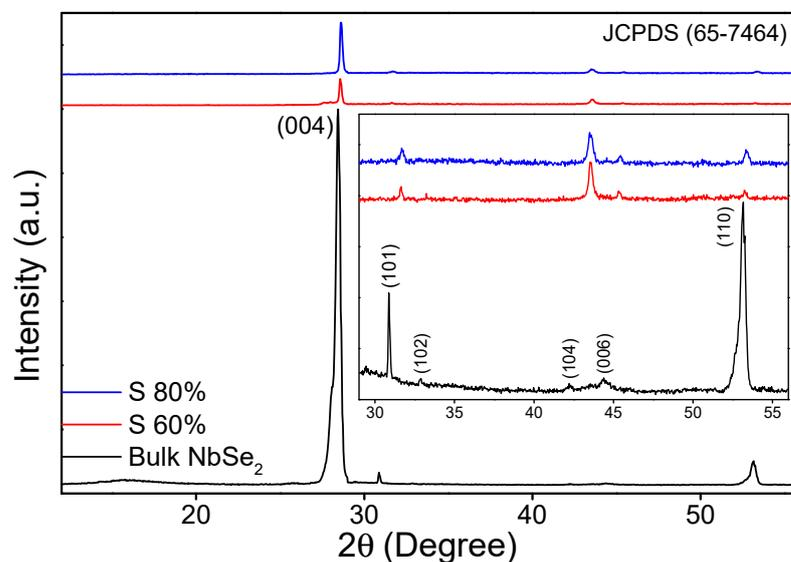
**Figure 1.** XRD of the NbSe<sub>2</sub> prepared via the liquid exfoliation method in comparison with the bulk (inset shows the peaks from 29 to 56 2θ).
