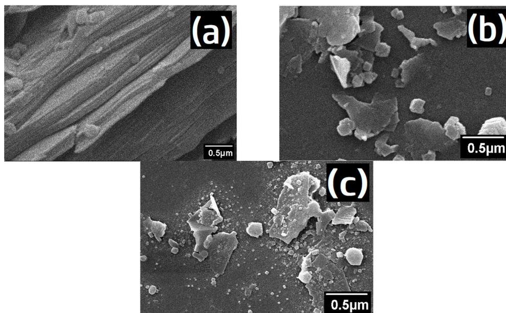
**Figure 2.** SEM images of the NbSe<sub>2</sub> prepared using the liquid exfoliation method compared to bulk. (a) Bulk; (b) prepared at 60%; and (c) prepared at 80%.
