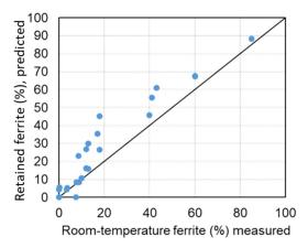
Figure 5. Comparison of predicted ferrite fraction by DICTRA simulations and measured values in [4].
