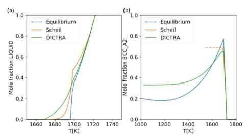
**Figure 4.** Comparison of cooling simulations under equilibrium condition, and under non-equilibrium conditions performed by Scheil and DICTRA. (a) Comparison of fraction of liquid during solidification; (b) comparison of  $\delta$ -ferrite fraction during continuous cooling.
