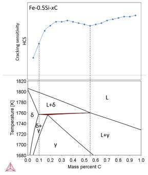
**Figure 3.** Relation between hot cracking susceptibility (HCS) and equilibrium phase diagram of the Fe-0.5Si-xC ( $x = 0.05 \sim 0.95$ , in wt.%) ternary system.
