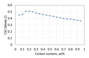
**Figure 2.** Cracking susceptibility coefficient (CSC, under mode 2 cooling condition) vs. carbon content for Fe-0.5Si-xC ( $x = 0.05 \sim 0.95$ , in wt.%) ternary system.
