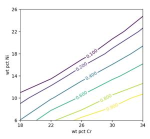
Figure 6. ICME-predicted "Schaeffler diagram".
