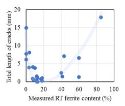
**Figure 1.** Total length of cracks vs.  $\delta$ -ferrite content measured at room temperature for 24 austenitic and austenitic-ferritic welds in [4].
