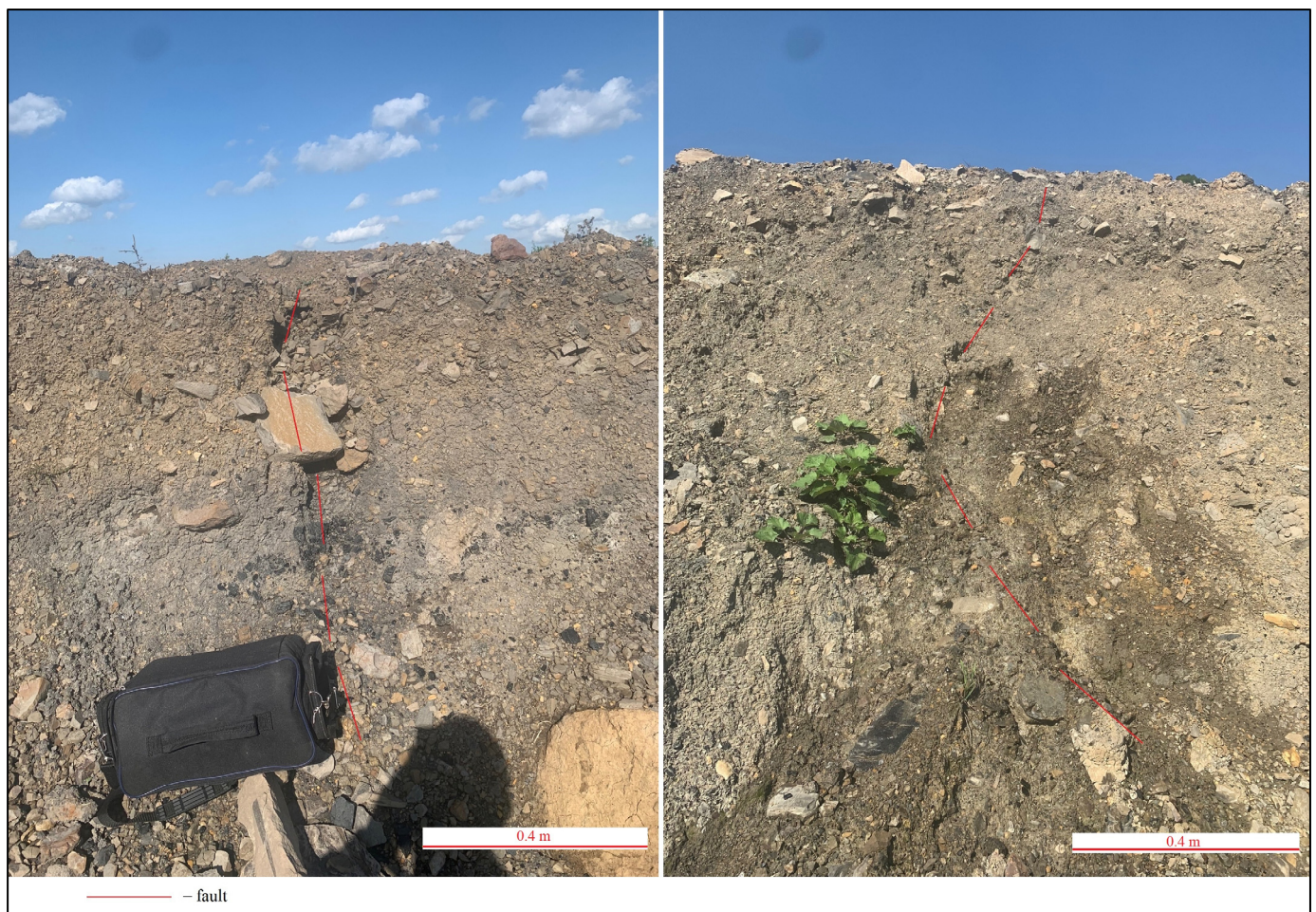
Figure 7. Faults on the overburden massif side. On the left without water outlet; on the right with groundwater outlet.
