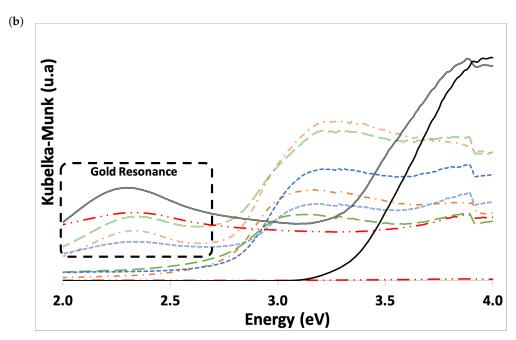
**Figure 4.** (a) DR UV-Vis spectra of the supports and the catalysts. (b) With the corresponding Tauc plots.
