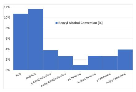
**Figure 6.** Dark test conducted under the following conditions: 4 h, 600 rpm, benzyl alcohol 24.7 mmol  $L^{-1}$ , 5 mL, pH = 2 ( $H_2SO_4$ ), 25 mg of catalyst (Substrate:Au = 48.6 [mol:mol]), no irradiation,  $P_{atm.}$ , without control of the temperature.
