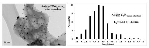
Figure 8. TEM and particles size distribution of  $Au@g-C_3N_{4(urea)}$  after photocatalytic test.
