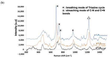
Figure 2. g-C<sub>3</sub>N<sub>4</sub> supports characterization: (a) XRD patterns. (b) Raman spectra.
