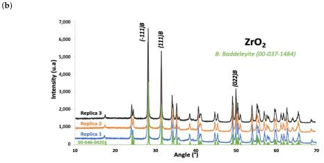
**Figure 1.** XRD patterns of the catalysts: (a) Au@TiO<sub>2</sub> replicas. (b) Au@ZrO<sub>2</sub> replicas.
