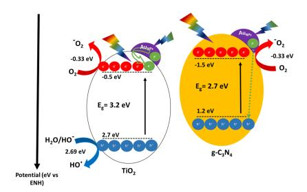
**Figure 9.** Illustration of the photoconduction through gold NPs supported on  $TiO_2$  and  $g-C_3N_4$ . The potential values were obtained from [57].
