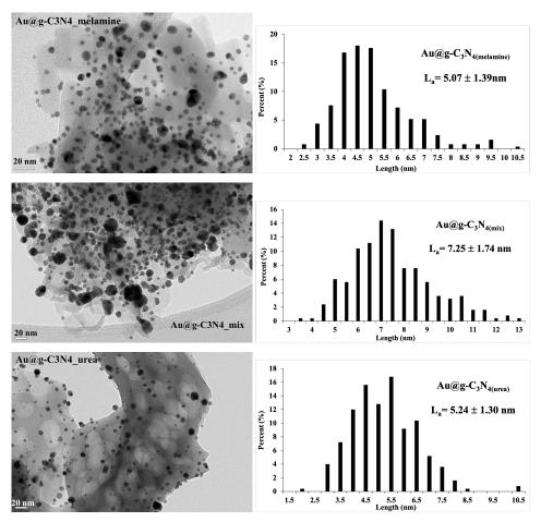
**Figure 5.** Typical TEM images and particle size distributions for Au NPs immobilized on the different precursors of g- $C_3N_4$ .
