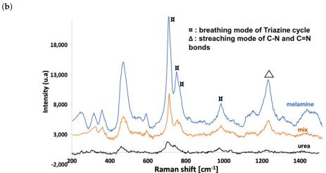
**Figure 3.** Au@g- $C_3N_4$  (a) XRD patterns with the g- $C_3N_4$  (black) and Gold NPs (red) phases. (b) Raman spectra.
