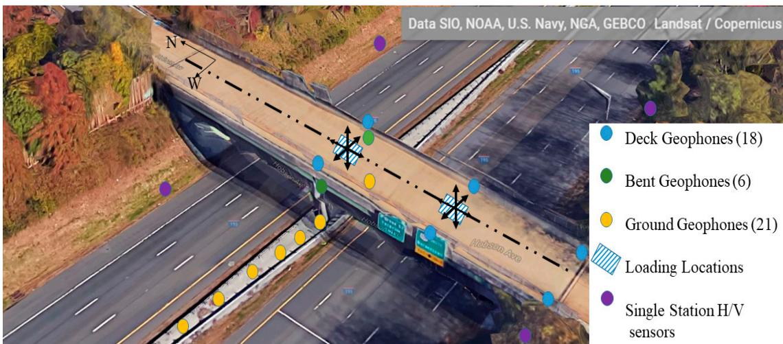
**Figure 7.** Overall sensor layout and T-rex loading positions. Reprinted with permission from Ref. [34].
