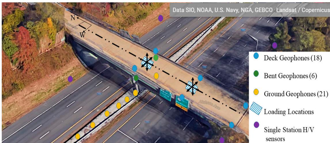
Figure 7. Overall sensor layout and T-rex loading positions. Reprinted with permission from Ref. [34].
