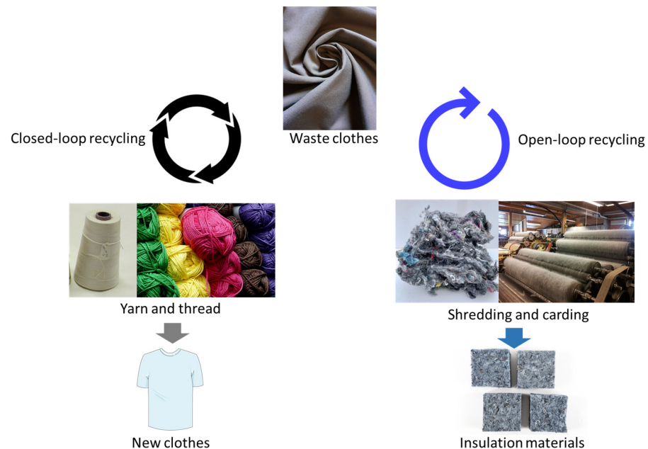
Figure 2. Closed-loop and open-loop mechanical recycling of textiles.
