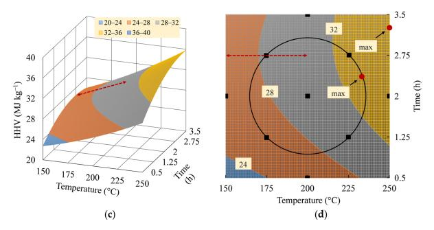
**Figure 7.** Raising-ridge contour of HHV: (a) 3D and (b) 2D plots of SB hydrochars; (c) 3D and (d) 2D plots of MA hydrochars.
