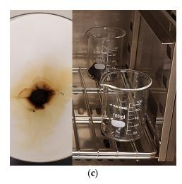
**Figure 1.** Schematic of hydrochar production. (a) Blending dried biomasses and deionized water in PTFE liner; (b) Activating HTC by inducting vessels thermally; (c) Separating slurry by filter paper before proceeding with final drying.
