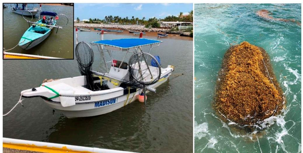
**Figure 2.** (Top Left) Littoral Collection Module (LCM) fitted onto a traditional “yola” boat. (Left) LCM fitted onto a small powerboat prior to the arms rotating the nets down into the water. (Right) A net of *Sargassum* filled by the LCM, floating in the water before it is towed away.
