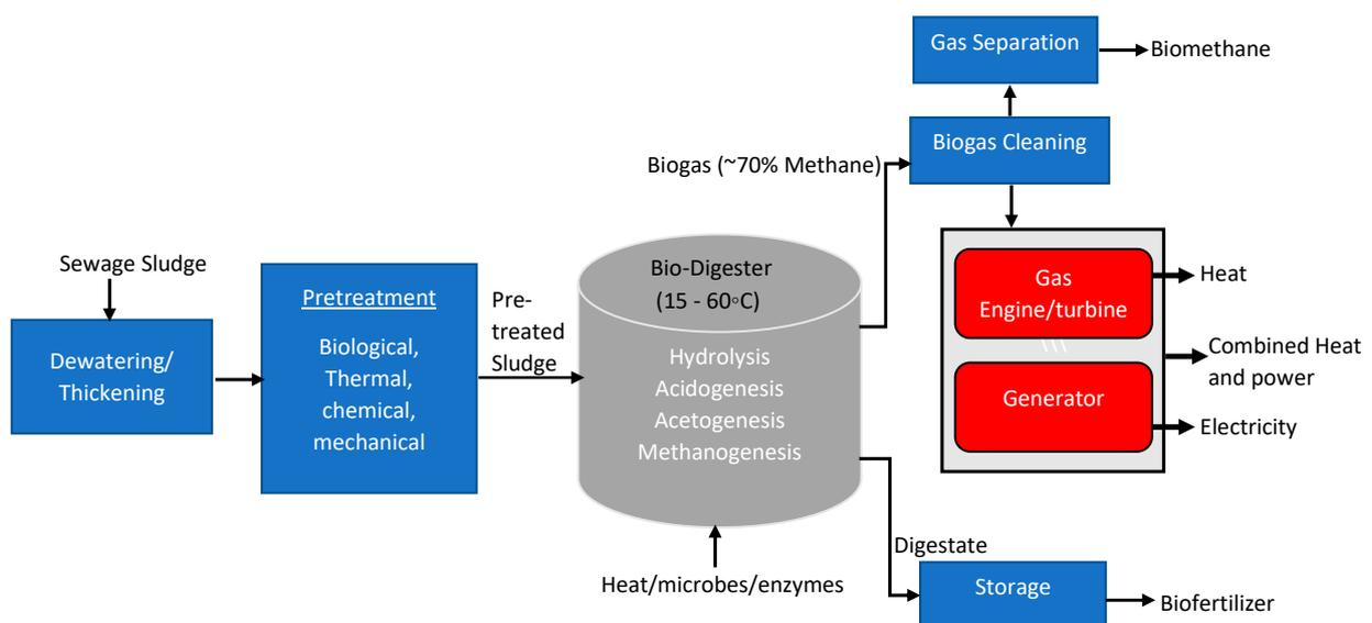
**Figure 2.** A schematic diagram of the sewage sludge valorisation process for biogas production.
