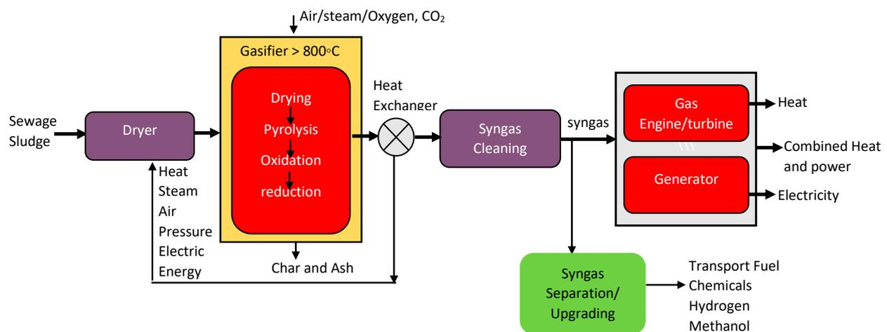
**Figure 3.** A schematic diagram of the sewage sludge valorisation process for syngas production.
