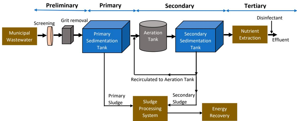
**Figure 1.** A summary layout of wastewater treatment steps for the production of sewage sludge and its valorisation to energy [5,45].
