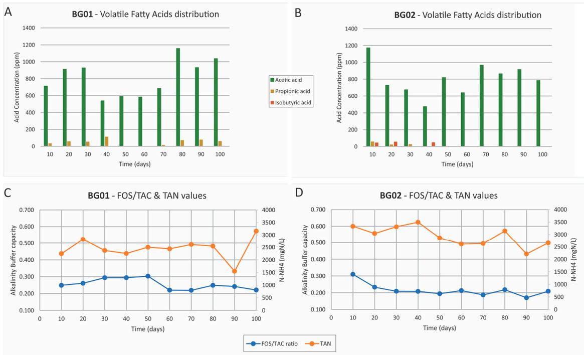
**Figure 2.** Volatile fatty acids distribution and FOS/TAC ratio in the two biogas plants; (A,B) Volatile fatty acids distribution in BG01 and BG02, respectively; (C,D) FOS/TAC ratio and TAN values in the BG01 and BG02 during Evogen biogas additive introduction. Day 50 is the interval day of Evogen supplementation.
