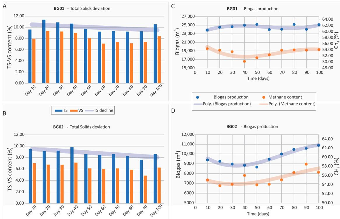
**Figure 1.** Total solids deviation and total biogas in the two biogas plants during the Evogen biogas additive administration; (A,B) Total solids deviation in BG01 and BG02, respectively, (C,D) Biogas production and methane content in BG01 and BG02, respectively. Day 50 is the interval day of Evogen supplementation.
