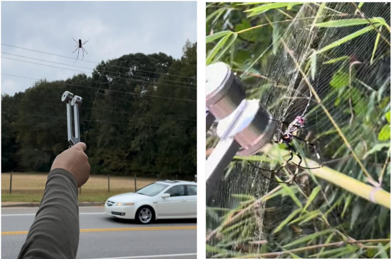
**Figure 2.** Photos of the prey simulation trials that elicited spider behavior. We used a tuning fork (128 hz) to simulate a buzzing insect hitting the web [25]. The fork was struck first to activate, then the handler gently touched it to the spider web at a point midway between the center and perimeter. Spiders can immediately sense the vibrations and either choose to attack the “prey” (right image) or not.
