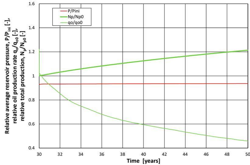
Figure 6. Scenario I. Reservoir pressure, oil rate, and total oil production.
