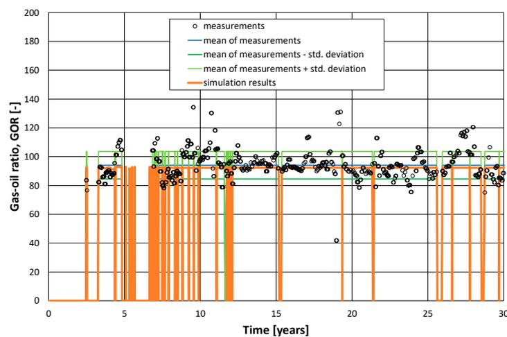
Figure 3. The result of the gas–oil ratio matching process for an example well.
