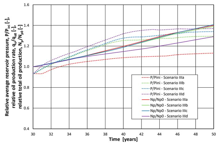
**Figure 16.** Scenarios IIIa, IIIb, IIIc, and IIId. Reservoir pressure and total oil production.
