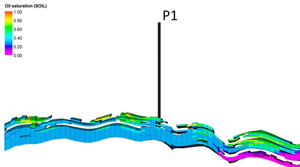
Figure 9. Scenario I. Distribution of oil saturation on a vertical cross-section along the main axis of the structure passing through the P1 well at the end of the forecast in 2042.
