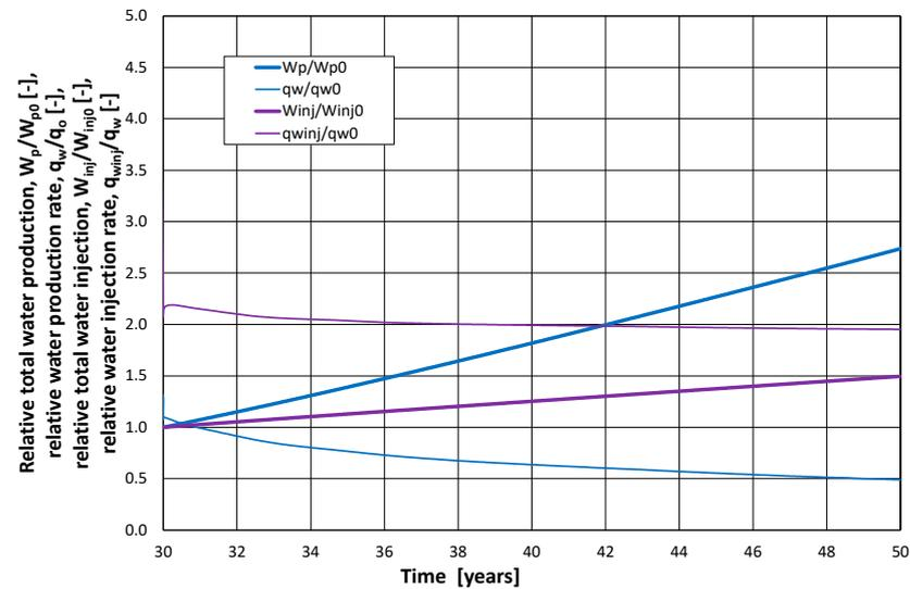
Figure 7. Scenario I. Rate and total water production and injection.
