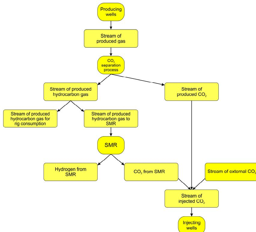
Figure 5. Diagram of gas flow in the project.
