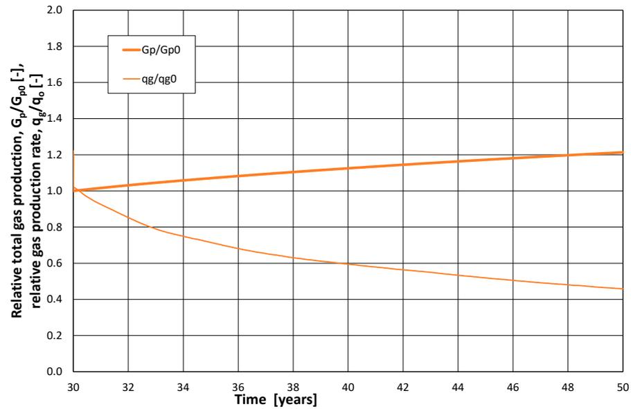
Figure 8. Rate and total gas production.
