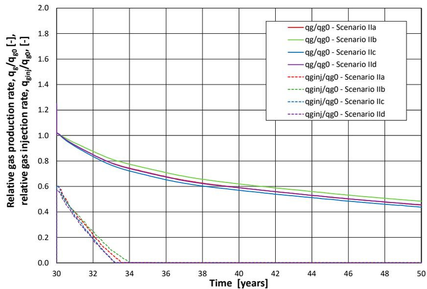
Figure 13. Scenarios IIa, IIb, IIc, IIId. Rate of gas production and CO<sub>2</sub> injection.
