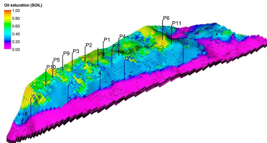
**Figure 11.** Scenario I. Distribution of oil saturation in the top layers of the reservoir at the end of the forecast in 2042.
