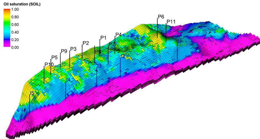
**Figure 10.** Distribution of oil saturation in the top layers of the reservoir at the beginning of the forecast in 2023.
