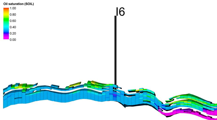
Figure 15. Scenario IIb. Distribution of oil saturation at the vertical cross-section along the main axis of the structure passing through the I6 well at the end of the forecast in 2042.
