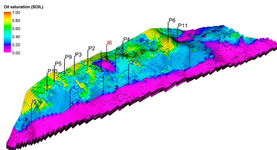
**Figure 19.** Scenario IIIa. Distribution of oil saturation in the top layers at the end of the forecast in 2042.
