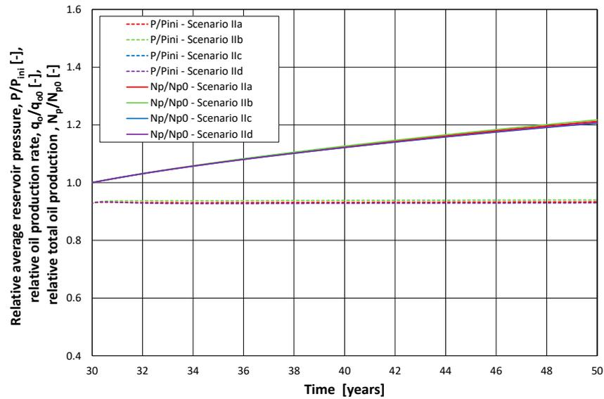
Figure 12. Scenario IIa, IIb, IIc, IIId. Reservoir pressure and total oil production.
