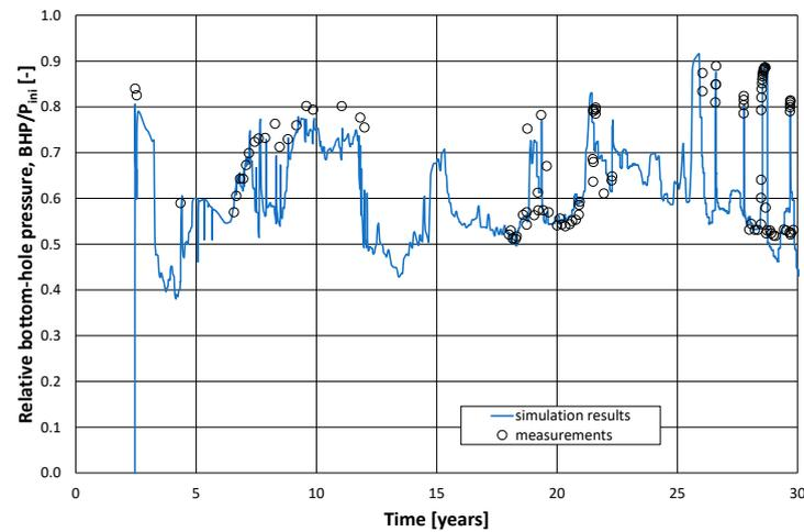
Figure 2. The result of the bottom pressure matching process for an example well.
