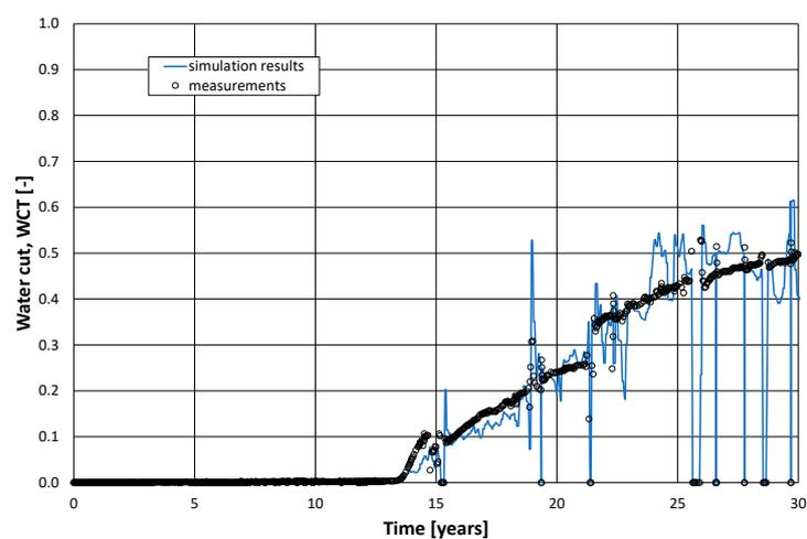
Figure 4. The result of the water cut matching process for an example well.
