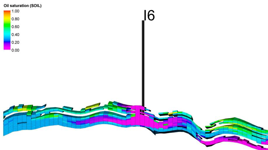
**Figure 18.** Scenario IIIa. Distribution of oil saturation at the vertical cross-section along the main axis of the structure passing through the I6 well at the end of the forecast in 2042.
