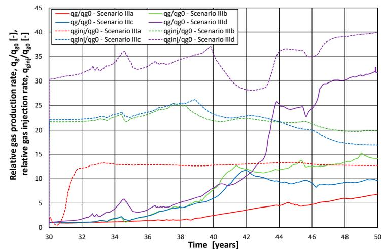
**Figure 17.** Scenarios IIIa, IIIb, IIIc, and IIId. Rate of gas production and CO<sub>2</sub> injection.
