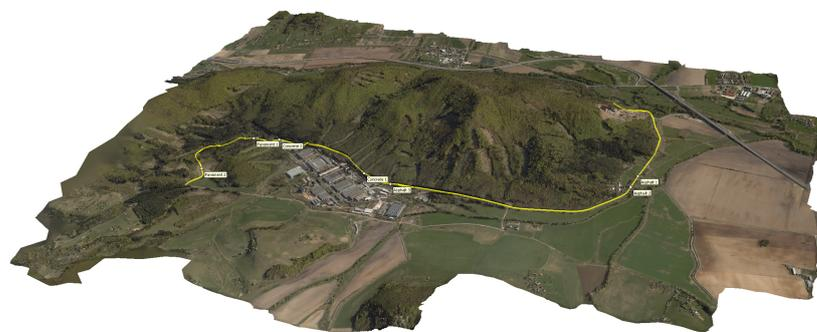
**Figure 4.** Example visualization of a three-dimensional forest road map with a resolution of 0.5 m and RGB coloration derived based on airborne laser scanning data.
