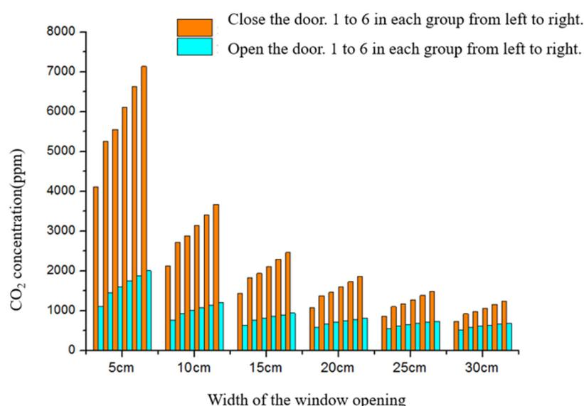
**Figure 9.** Simulation statistics of daytime working conditions in the dormitory. The X-axis means the opening width of the window, and the height of the window is always 1.3 m.
