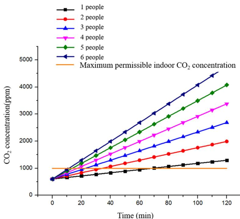
**Figure 8.** Changes in indoor CO<sub>2</sub> concentrations for different numbers of occupants when doors and windows are closed.
