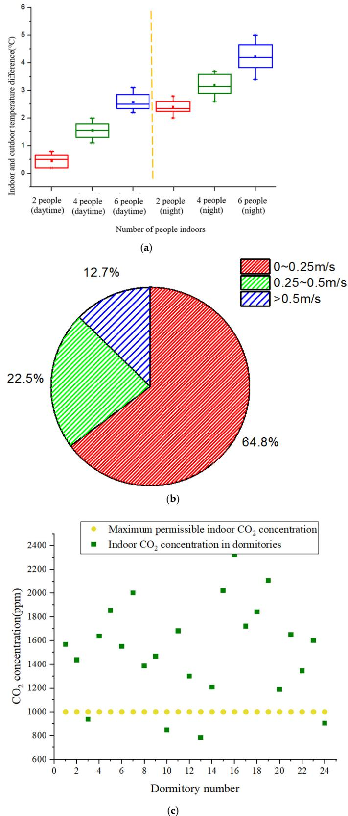
**Figure 6.** Measurement of indoor and outdoor parameters of dormitory in transitional season. (a) Actual measurements of indoor and outdoor temperatures in a typical dormitory. (b) Actual measurements of outdoor wind speed around a typical dormitory. (c) Actual measurements of indoor CO<sub>2</sub> concentrations in different dormitories.
