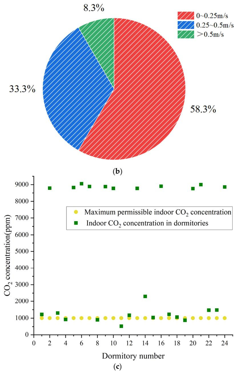
**Figure 7.** Actual measurements of indoor and outdoor parameters in dormitories during winter seasons. (a) Actual measurements of indoor and outdoor temperatures in a typical dormitory during winter. (b) Actual measurements of outdoor wind speed around a typical dormitory during winter. (c) Actual measurements of indoor CO<sub>2</sub> concentrations in different dormitories during winter.
