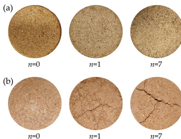
**Figure 6.** Pictures of soil samples with varying numbers of cycles ( $n$ ). (a) sandy clay soil; (b) clay soil that is powdery.
