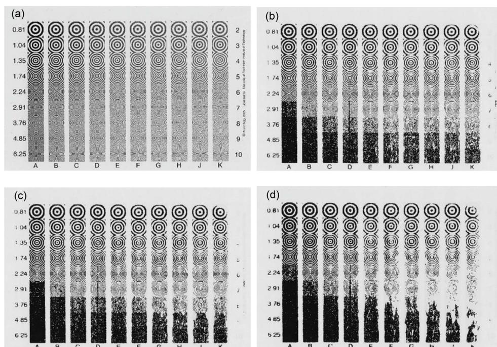
**Figure 10.** Bitmap images of metalized elements after cold foil transfer: (a) EP reference; (b) layer generate with speed 0.300 m/s; (c) layer generate with speed 0.240 m/s; (d) layer generate with speed 0.159 m/s.
