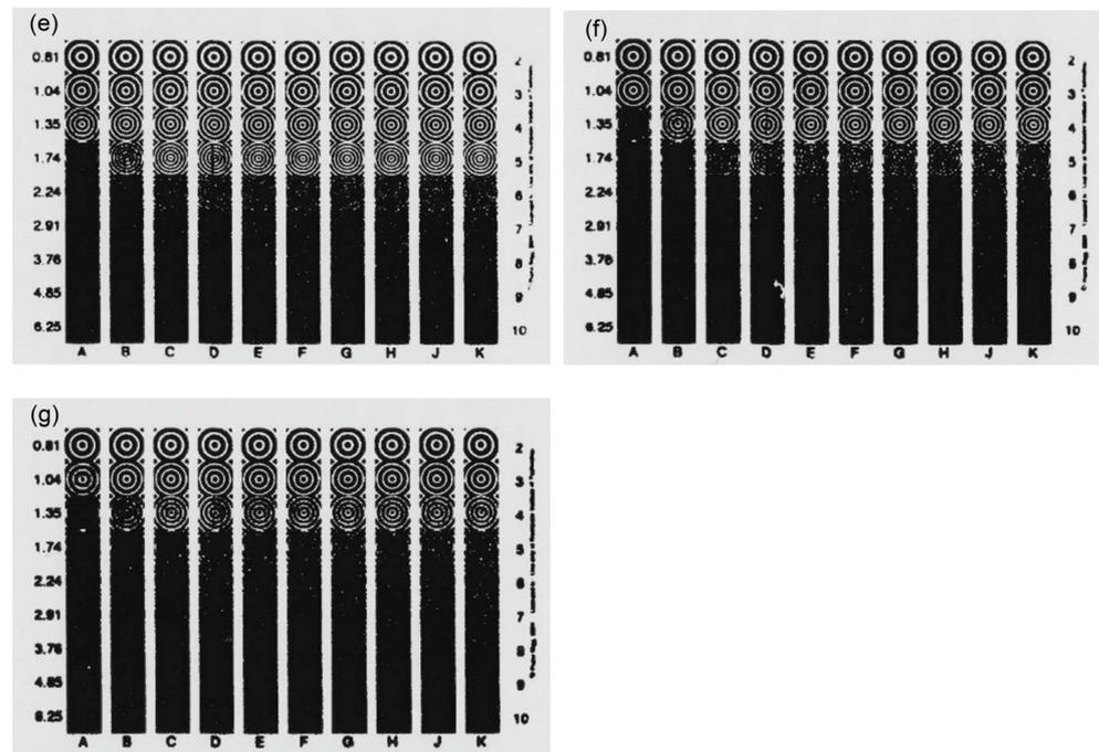
**Figure 8.** Bitmap images of metalized elements after cold foil transfer: (a) EP reference; (b) layer with 21 μm; (c) layer with 29 μm; (d) layer with 36 μm; (e) layer with 43 μm; (f) layer with 51 μm; (g) layer with 58 μm.
