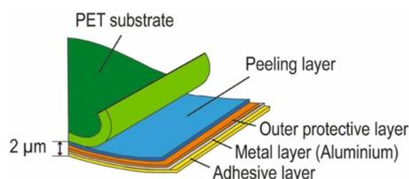
**Figure 1.** Typical composition of metalized foils for cold foil application [7].
