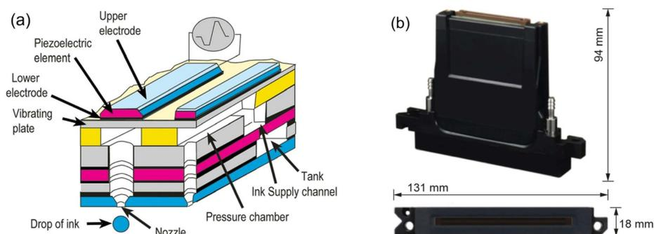
**Figure 4.** Construction of an inkjet piezo nozzle for applying UV-cured ink (adhesive): (a) schematic view; (b) KM series head KM1024i [18].
