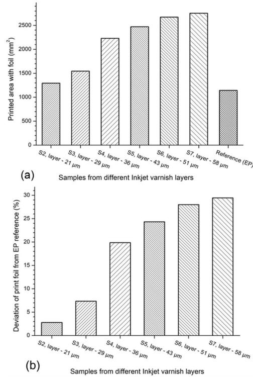
**Figure 7.** Results of the resolution test of samples created by varying the application varnish with a JET Varnish 3DS machine: (a) printed area in mm<sup>2</sup>; (b) deviation between samples and EP reference.
