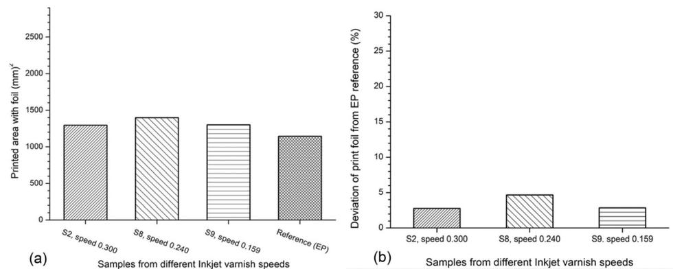
**Figure 9.** Sample resolution test results obtained by varying the printing speed of the JET Varnish 3DS machine: (a) printed area in mm<sup>2</sup>; (b) deviation between samples and EP reference.
