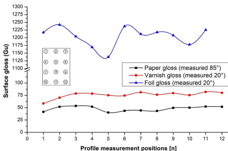
**Figure 6.** Gloss profiles of the surfaces used in the experiment (cardboard, cardboard + varnish, cardboard + varnish + foil).
