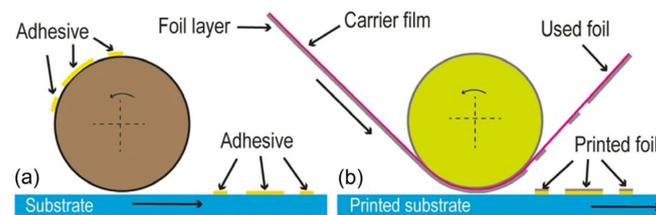
**Figure 3.** Principles of hot foil printing: (a) vertical hot foil printing machine; (b) roll-on hot foil printing machine [8].
