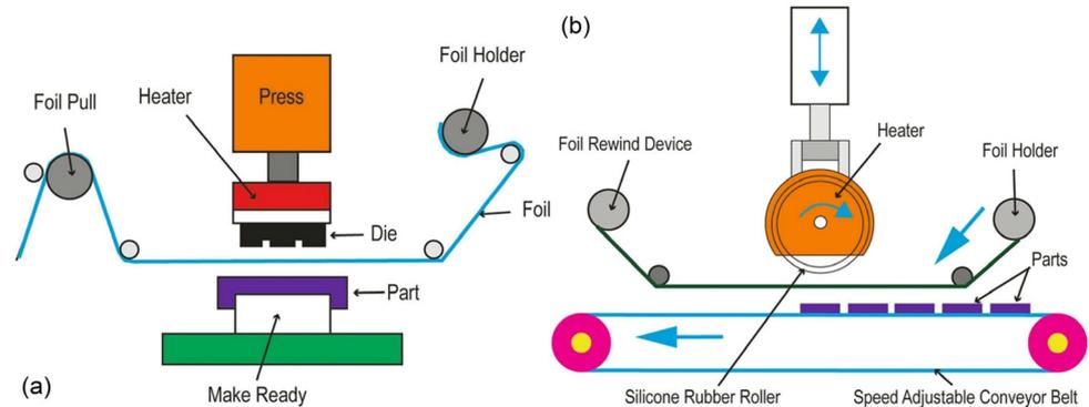
**Figure 2.** Principles of and tools for hot foil printing: (a) vertical hot foil printing machine; (b) roll-on hot foil printing machine [10].
