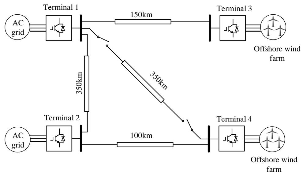
Figure 12. A 4-terminal MTDC network connected to offshore wind farm.
