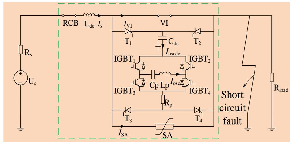
Figure 5. The simulation model of DC interruption.
