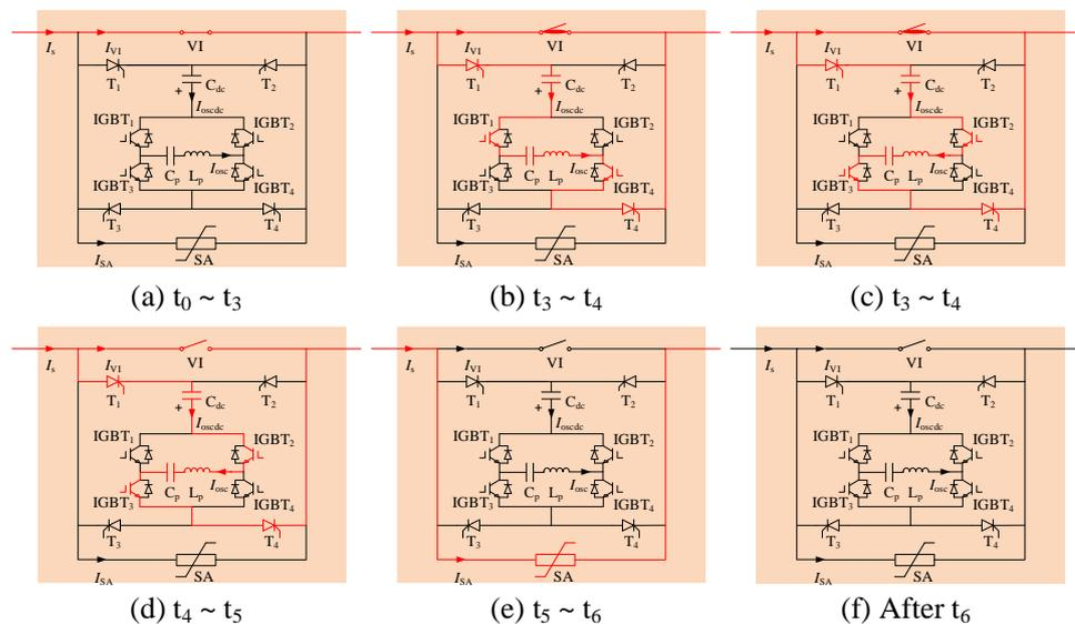
Figure 2. The working sequence of interruption.
