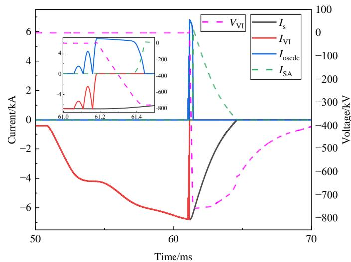
**Figure 16.** Simulation results of CB at the negative pole of terminal 4.
