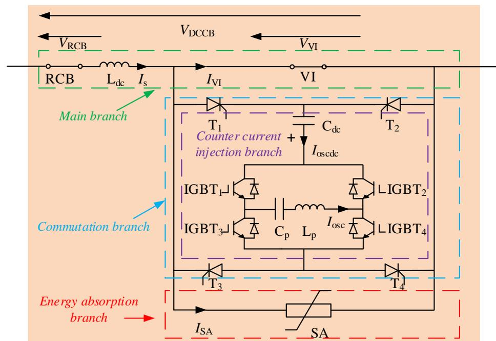
**Figure 1.** Schematic of the novel DC circuit breaker.
