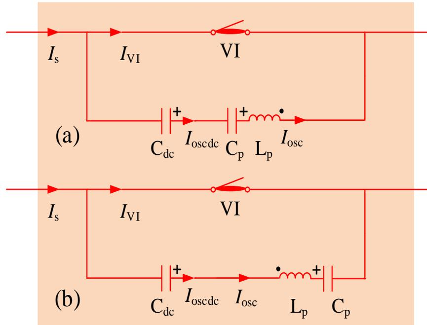
**Figure 4.** Illustration of oscillation process in commutation branch; (a) oscillation circuit in first half-cycle of oscillation; (b) oscillation circuit in second half-cycle of oscillation.
