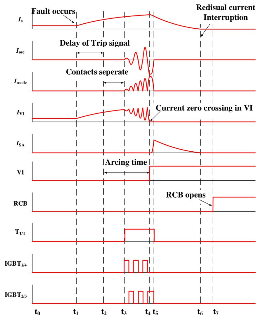
**Figure 3.** The waveform and status during the interruption.
