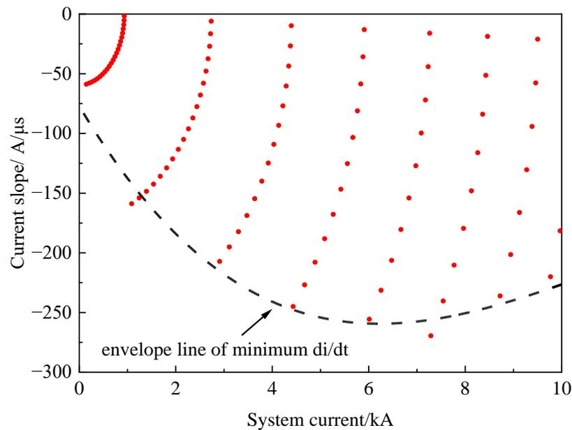
Figure 8. Current slope with regard to different system currents.
