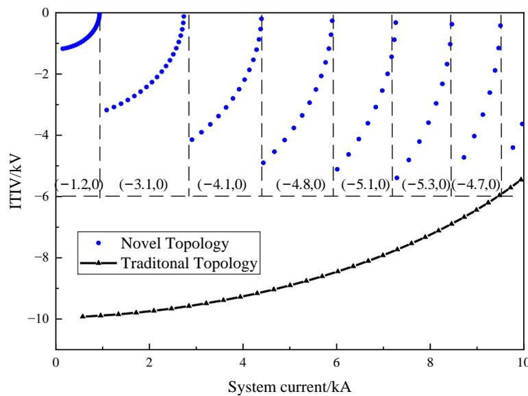
Figure 11. Comparison of ITIV between the two topologies.
