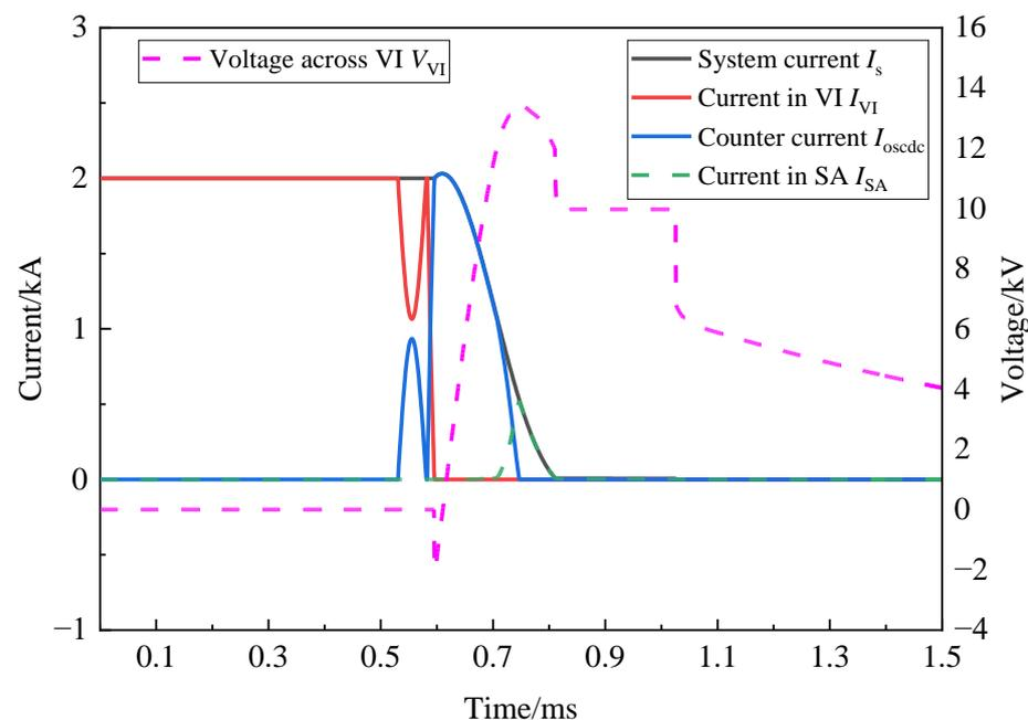
**Figure 6.** Simulation results of rated current interruption.
