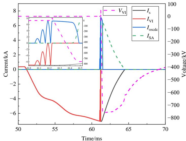
Figure 14. Simulation results of CB at the negative pole of terminal 1.
