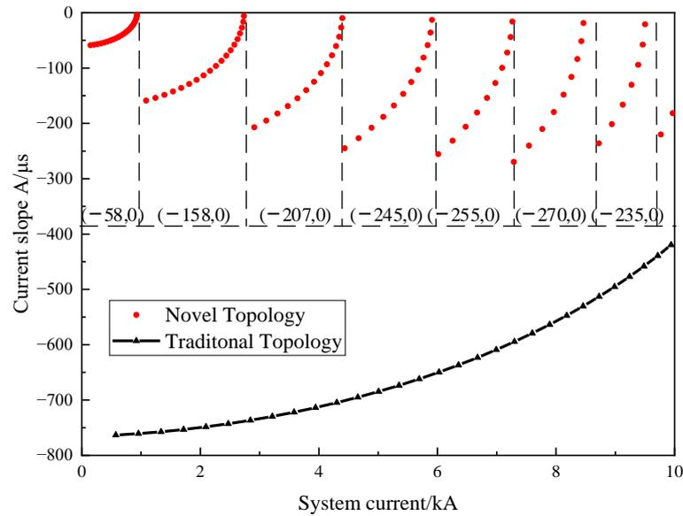
Figure 10. Comparison of  $di/dt$  between the two topologies.
