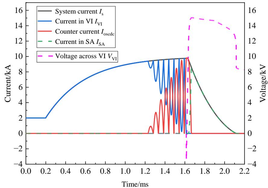
Figure 7. Simulation results of fault current interruption.
