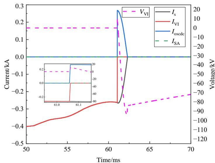
**Figure 13.** Simulation results of CB at the positive pole of terminal 1.
