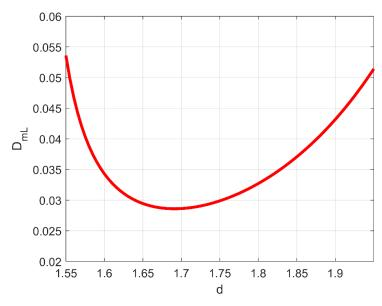
**Figure 1.** Normalized longitudinal macrodispersion coefficient in evolving-scale, anti-persistently correlated (0 < b < 1) log-conductivity distributions as a function of the corresponding (single) fractal dimension (Equation (3), from [3]).
