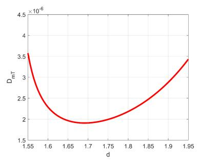
**Figure 2.** Normalized transverse macrodispersion coefficient in evolving-scale, anti-persistently correlated (0 < b < 1) log-conductivity distributions as a function of the corresponding (single) fractal dimension (Equation (4), from [3]).
