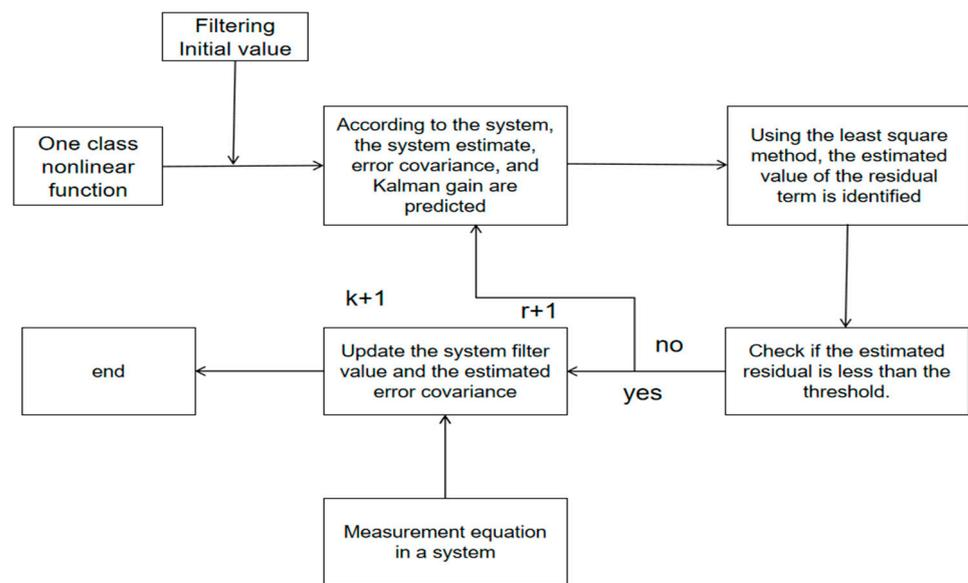
**Figure 1.** The flow chart represents the relationship between the nonlinear system and the Kalman filter, and the updating process of the REKF.
