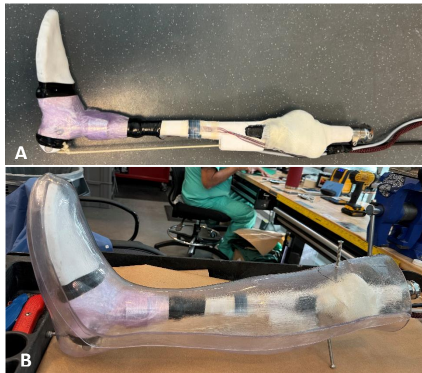
Figure S5: (A) lateral view of completed musculoskeletal apparatus with joint capsule and (B) musculoskeletal apparatus in the 50th percentile male leg mold with pin alignment prior to silicone pour.
