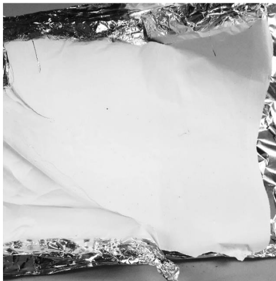
Figure S1. Digital photograph of electrospun NaCM- iB nanofiber mat.
