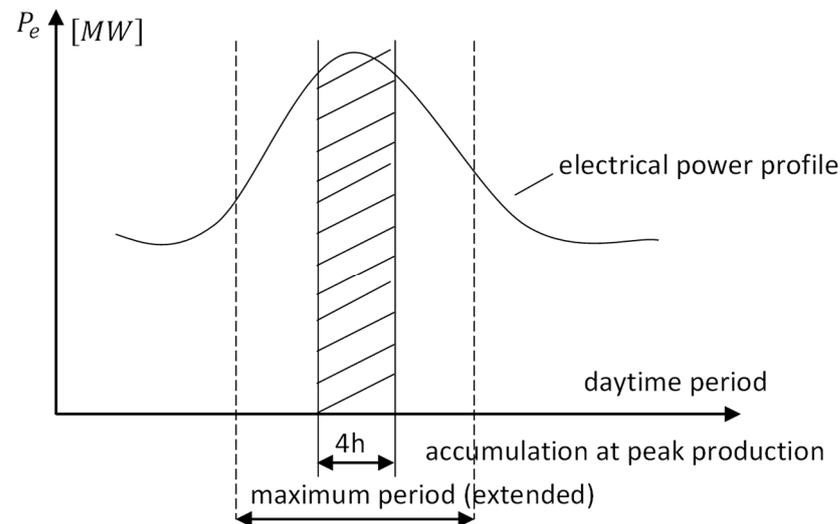
**Figure 4.** The period of electricity consumption from renewable sources between heating the hot water storage.
