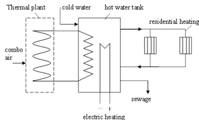
**Figure 6.** The scheme of electricity accumulation in hot water in a system equipped with a heat accumulator connected to the heating system.
