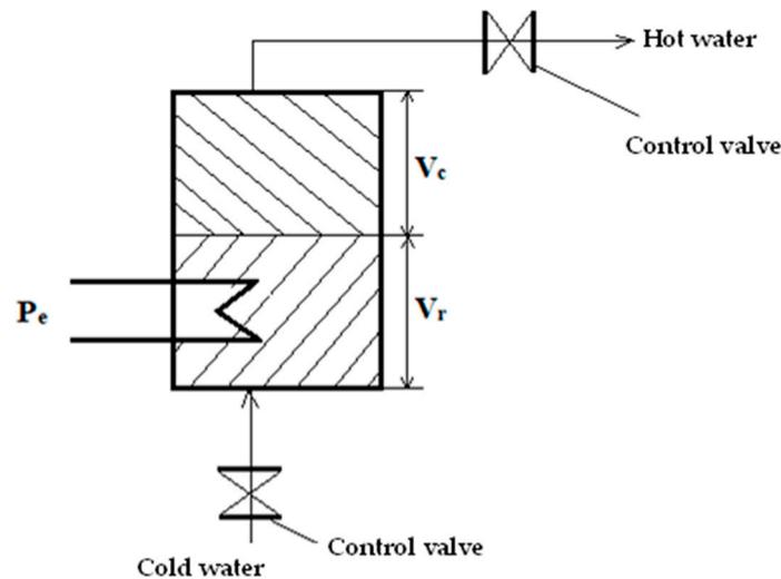
**Figure 5.** Scheme of the dynamic operation of the hot water accumulator.
