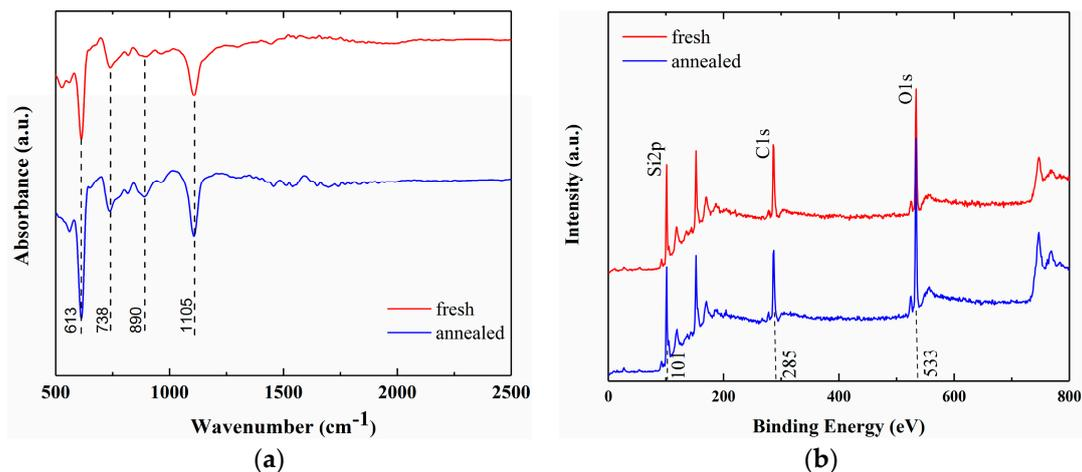
Figure 7. Spectra of (a) FTIR and (b) XPS obtained from freshly prepared and annealed sample.
