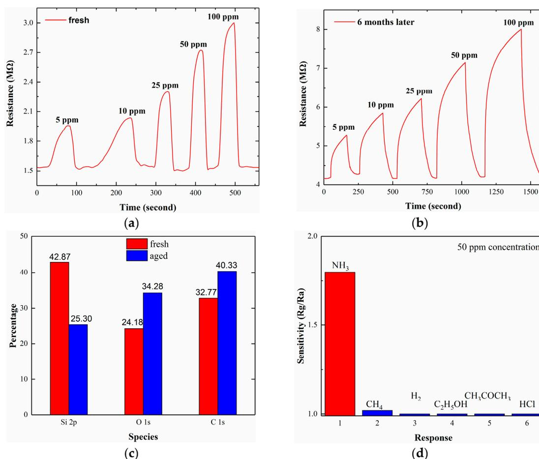
**Figure 3.** Dynamic response of (a) Fresh sample and (b) sample stored in air for 6 months versus  $\text{NH}_3$  concentrations ranging from 5 to 100 ppm. (c) The proportion of Si 2p, O 1s and C 1s species in the sample before and after ageing. (d) Selectivity of the sensor for 50 ppm  $\text{NH}_3$ ,  $\text{CH}_4$ ,  $\text{H}_2$ ,  $\text{C}_2\text{H}_5\text{OH}$ ,  $\text{CH}_3\text{COCH}_3$  and HCl.
