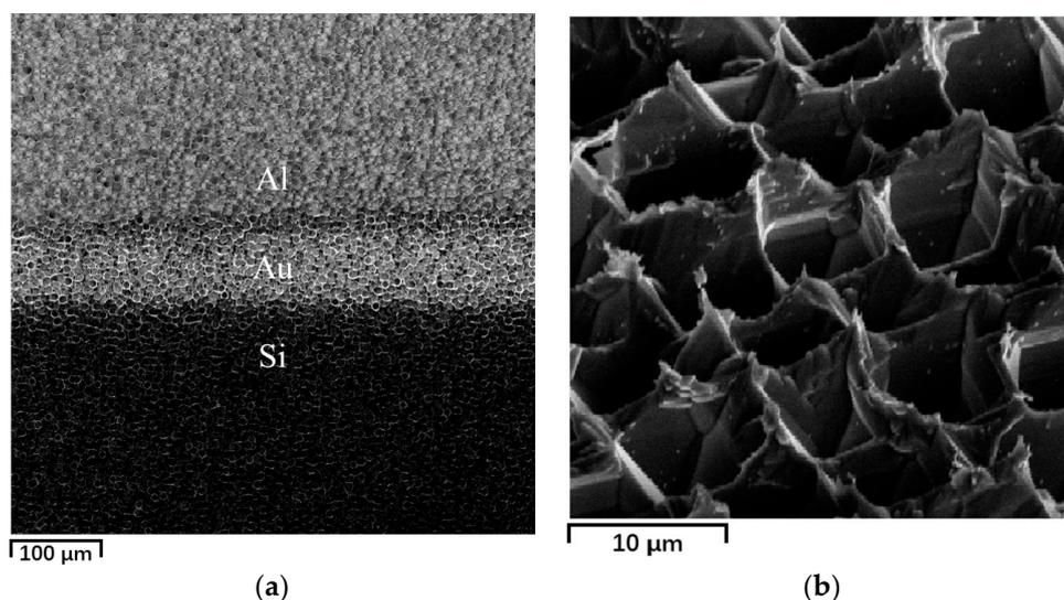
**Figure 5.** SEM micrographs of the treated sensors. (a) Short-circuited electrode (viewed at  $0^\circ$ ). (b) Surface morphology after annealing (viewed at  $45^\circ$ ).
