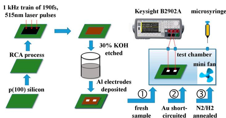
**Figure 2.** Schematic diagram of sensor fabrication and sensing test system.
