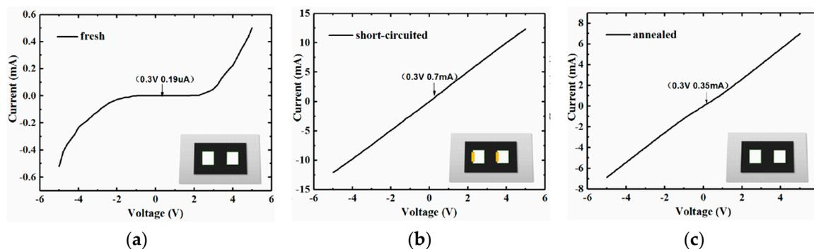
Figure 4. I-V curves of (a) freshly prepared, (b) short-circuited and (c) annealed sensors.
