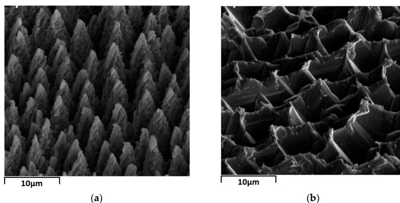
**Figure 1.** SEM micrographs (viewed at  $45^\circ$ ) of laser-textured silicon surface (a) before and (b) after alkaline etching.
