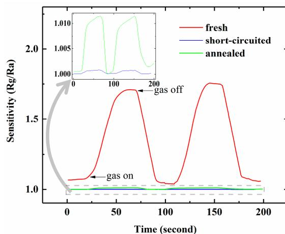
**Figure 6.**  $\text{NH}_3$  response of freshly prepared, short-circuited and annealed sensors at 50 ppm concentration.
